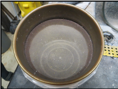
Fig 8: 1 mm mesh sieve
