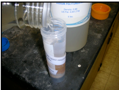
Fig. 10: Grain Immersion in LMT
