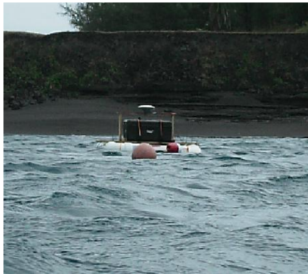
Figure 1. Water level buoy off a volcanic sand beach in the Mariana Islands. This manually deployed water level buoy was used to accurately determine water levels at the time of imaging.
