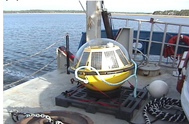
Figure 1. TRIAXYS™ buoy awaiting deployment from R/V Savannah (Skidaway Institute of Oceanography). Railroad wheel anchor in foreground; elastic mooring section to right in photo.
