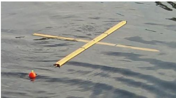
Figure 1. The reference cross for imaging small waves in creeks and rivers. The markings are one foot apart, and the float, to record vertical motions, is one foot behind the cross leg.
