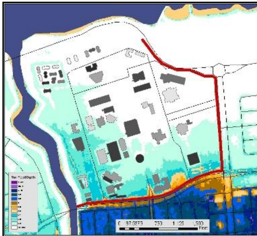
Figure 4.2: Limits of campus levee/floodwall (protection from 100 year flood event)
