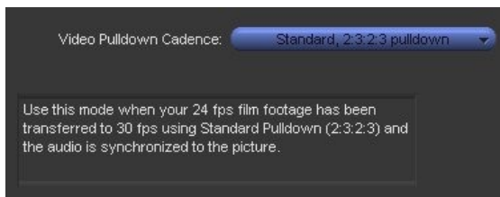
Figure 7. The Video Pulldown Cadence option in the Film and 24P Project settings dialog.
