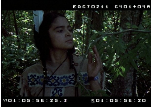
Figure 2. A frame of video showing key number, 30, and 24 fps timecode values “burned in”.
