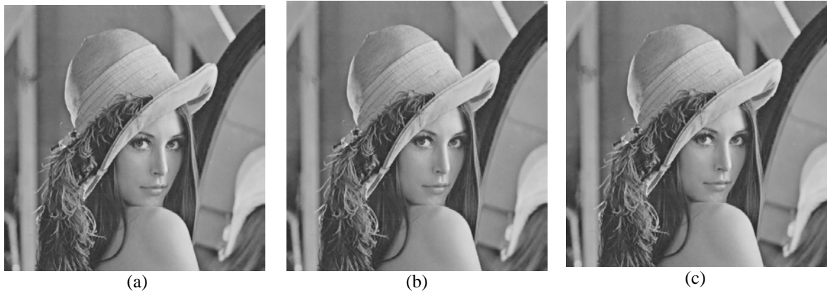
Figure 8: Visual Quality Comparison using Lens Wall image of Kwok's algorithm with different numbers of truncated coefficients. From left to right: m = 4 , m = 8 , and m = 40
