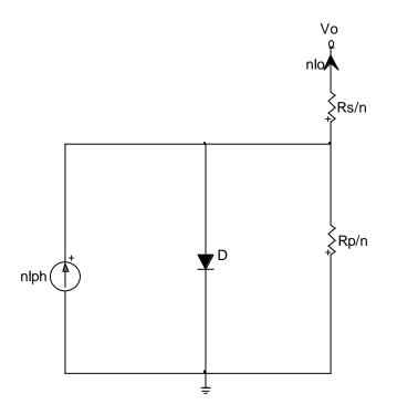
Figure 3.21 Equivalent model of PV panel with n cells in parallel.
