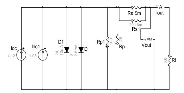
Figure 4.13: Parallel connection of solar cell model
