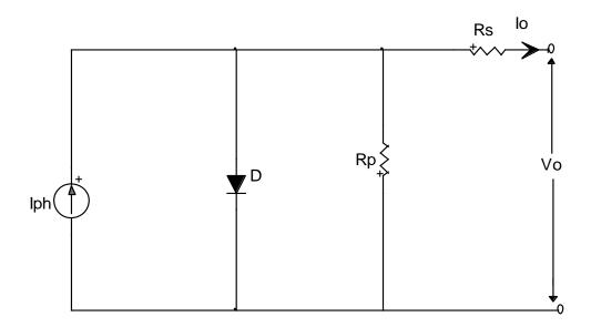
Figure 3.3: Single Solar cell circuit
