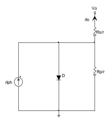
Figure 3.17: Model of a PV panel with r cells in parallel
