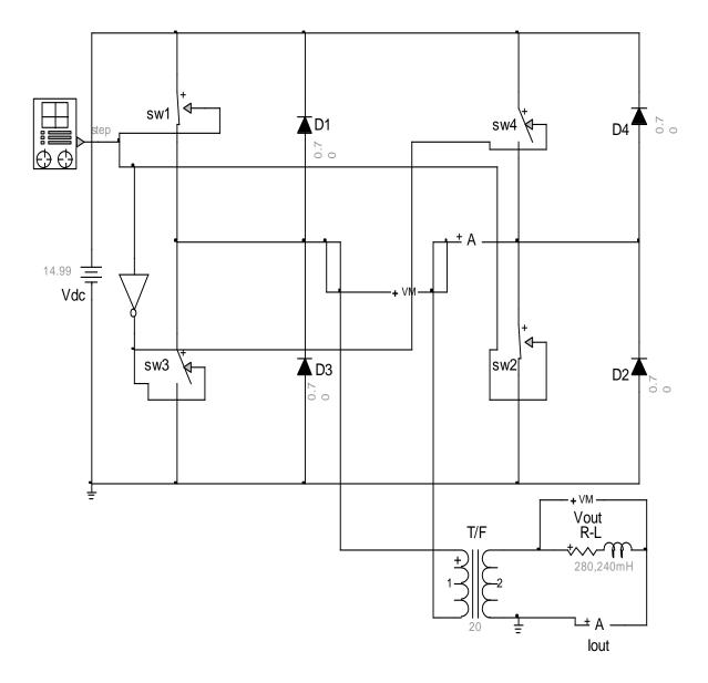
Figure 4.11: Solar series inverter connected to transformer
