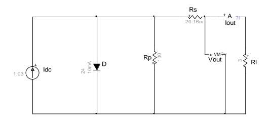
Figure 4.1: Single solar cell circuit
