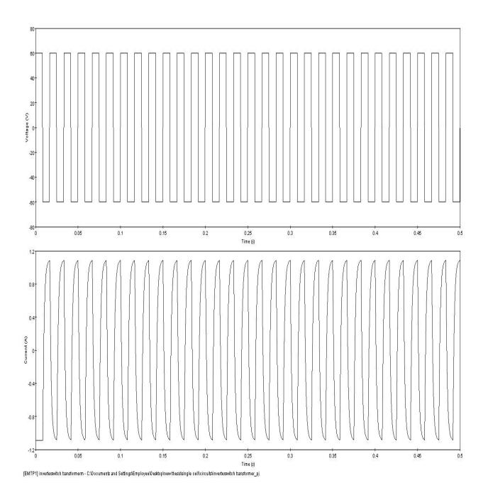
Figure 4.6: Voltage and current at transformer secondary side
