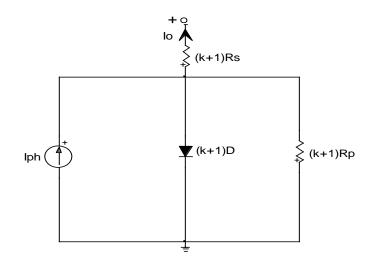
Figure 3.9: Model for (k+1) solar cells connected in series
