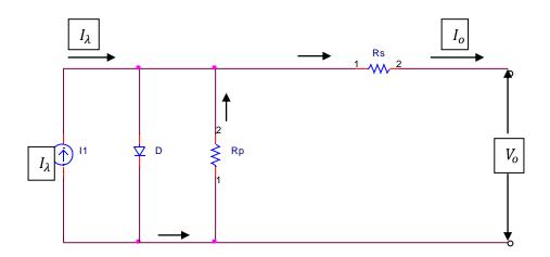
Figure: 3.1: Solar cell circuit
