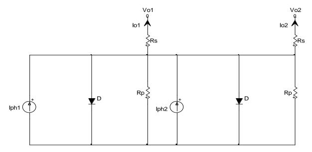
Figure 3.14: Model for two solar cells connected in parallel
