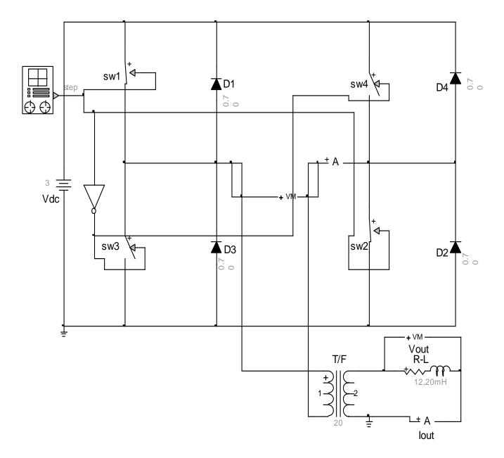
Figure 4.17 Solar parallel inverter connected to the transformer
