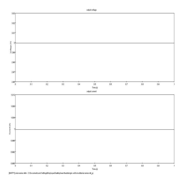
Figure 4.2: Output voltage and output current wave forms of single solar cell from EMTP
