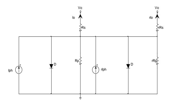
Figure 3.20: Model of a PV panel with r cells and 1 cell.
