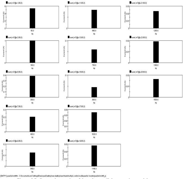
Figure 5.7: Current harmonics of the solar parallel connection model
