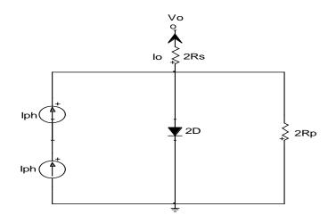
Figure 3.7: Modified Two Solar cells circuit
