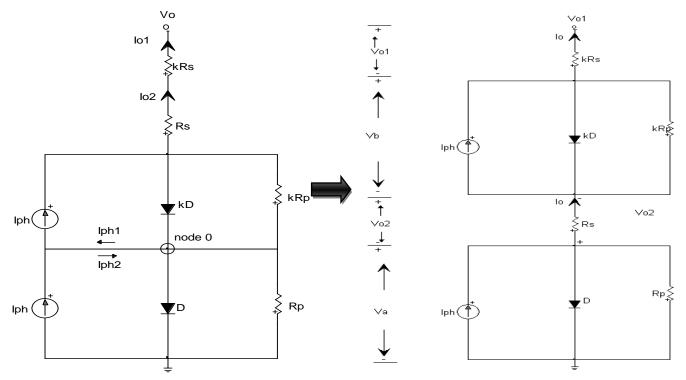
Figure 3.11: PV panel connected with k solar cells and 1 solar cell
