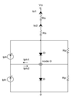
Figure 3.6: Modified Two Solar cells circuit
