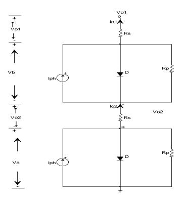
Figure 3.5: Two Solar cells connected in series
