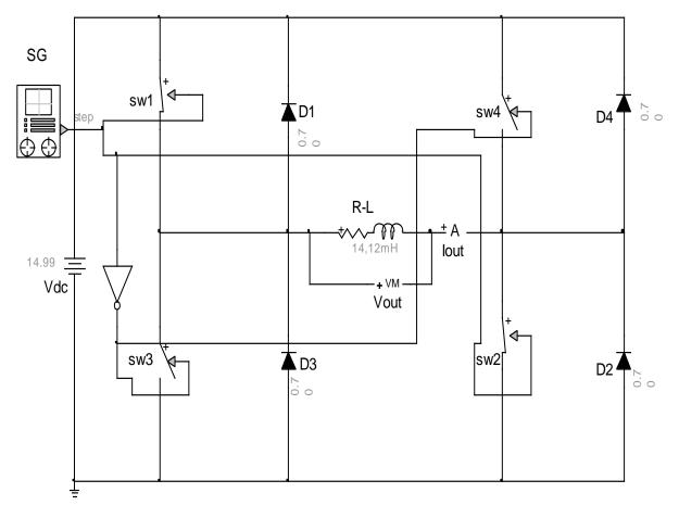
Figure 4.9: Series of solar cells connected to Inverter
