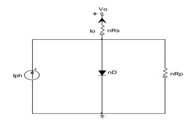
Figure 3.12: Equivalent model of a PV panel with identical n cells in series.
