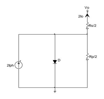
Figure 3.16: Model for Two solar cells connected in parallel.
