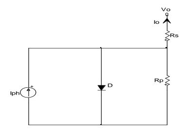
Figure 3.4: Modified Single Solar cell circuit
