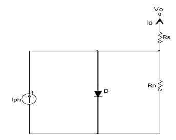
Figure 3.13: Model for single solar cell
