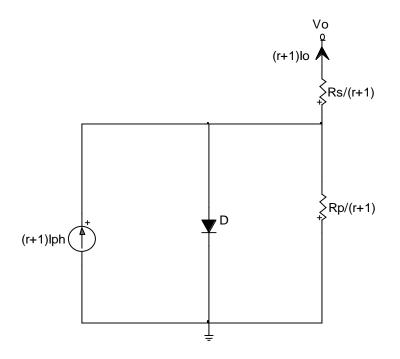
Figure 3.18: Model of a PV panel with (r+1) cells in parallel
