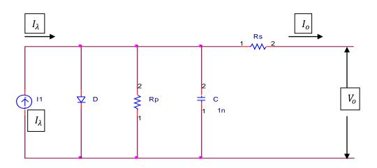
Figure: 3.2: Equivalent model and parameters for PV panel
