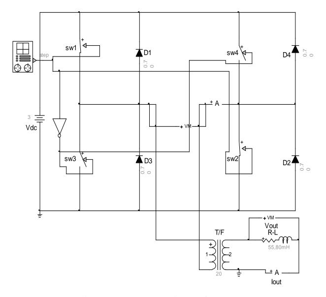
Figure 4.5: Inverter connected to Transformer
