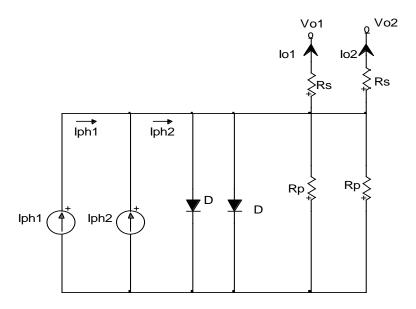
Figure 3.15: Modified model for two solar cells connected in parallel.
