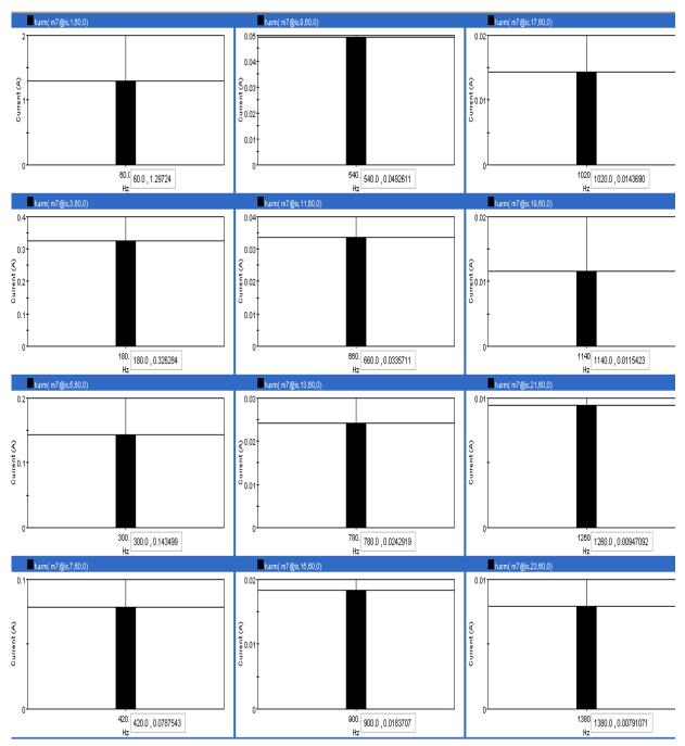
Figure 5.4: Current harmonic values for solar series connection model
