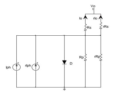
Figure 3.19: Model of a PV panel with r cells and 1 cell.
