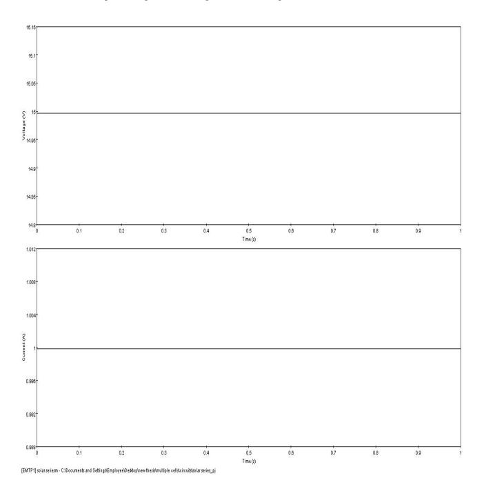
Figure 4.8: Output voltage and output current when solar cells are connected in series
