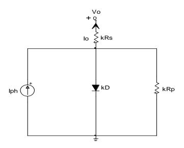
Figure 3.8: Model for k solar cells connected in series
