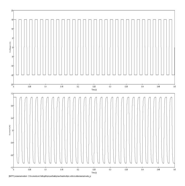
Figure 4.10: Output voltage and current with solar series cells connected to inverter
