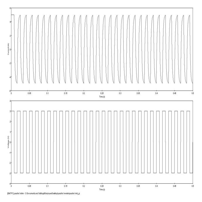
Figure 4.16: Output current and voltage of the parallel connected solar cell inverter
