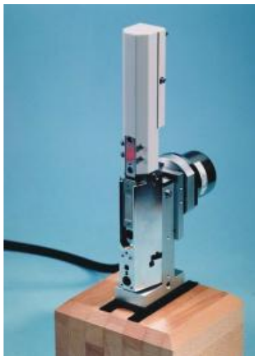
Figure 3.8: Programmable Receiving Slit (from [102])
