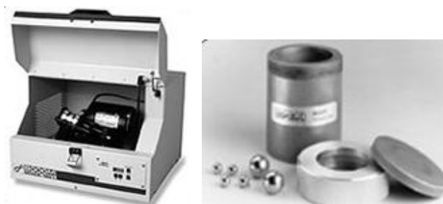
Figure 3.1: Mixer Mill and Hardened Steel Vial
