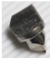
Figure 3.13: Diamond Indenter with Berkovich Geometry (from [113])
