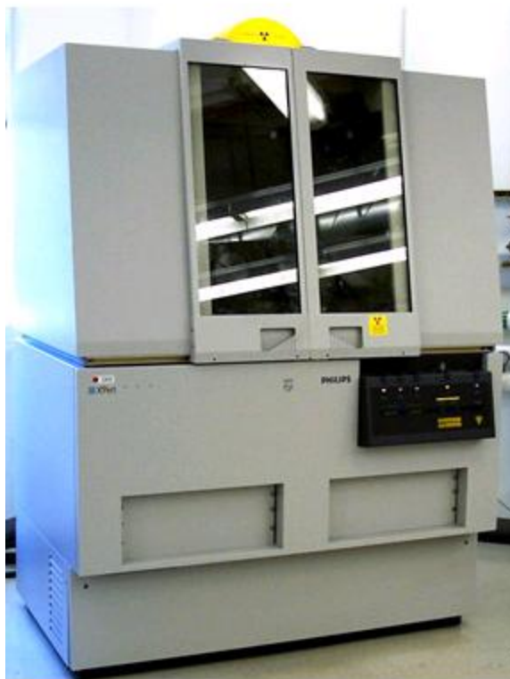
Figure 3.2: PW 3040/60 X'Pert Pro X-ray Diffraction System (from [102])
