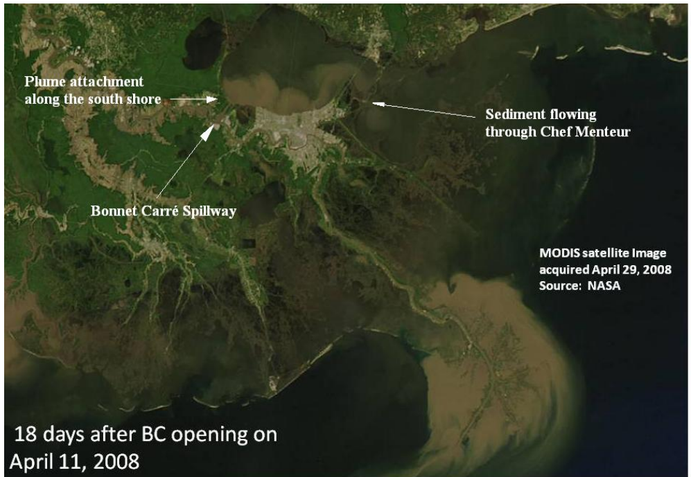
Figure 5.88: Satellite image on April 29 th , 2008 showing the sediment propagation due to the 2008 opening of the Bonnet Carré Spillway.
