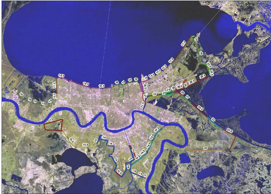
Figure 25 USACE 100 year level of protection levee heights
