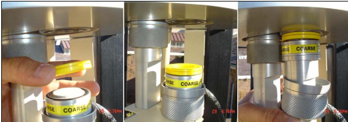
Figure 5: Placing of the Coarse Particles Filter in the Dichotomous Sampler
