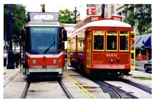
Source: RTA 2007a. Note: Streetcar vehicle on right (2000 Series Von Dullen) shown next to a modern style LRT vehicle on left.
