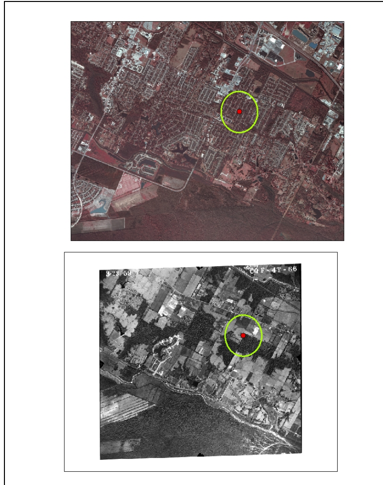
Figure 2.2 Illustration of “current” and “historic” sites. Both are in the same geographic location, but the current site is plotted on a DOQQ and the historic site is plotted on a historical aerial photograph that has been georeferenced and rectified.
