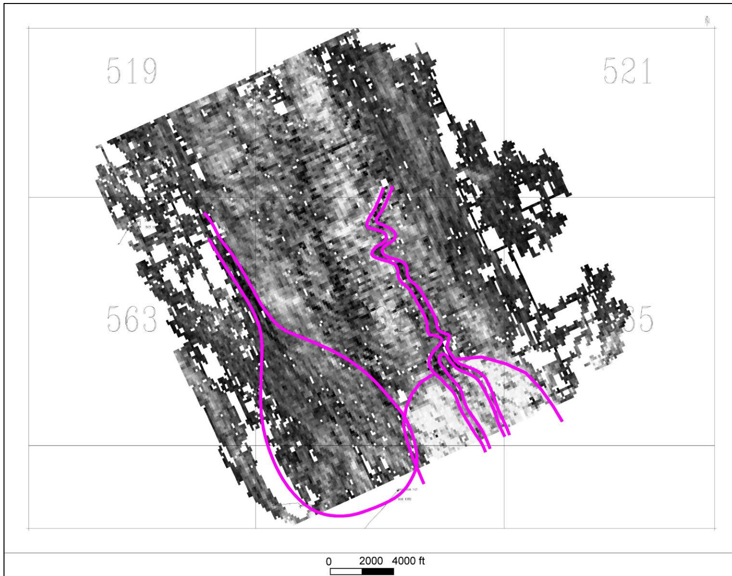
Figure 18—RMS amplitude extraction from the upper light blue horizon in Fig. 17, which is at a depth of approximately 8900 ft. The left lobe is interpreted as a channel/fan transition zone due to the dendritic channel patterns emanating from the channel source. The sinuous channel on the right bifurcates into an area that is possibly a channel/lobe transition zone. These systems are Pleistocene on the basis of available biostratigraphic data.
