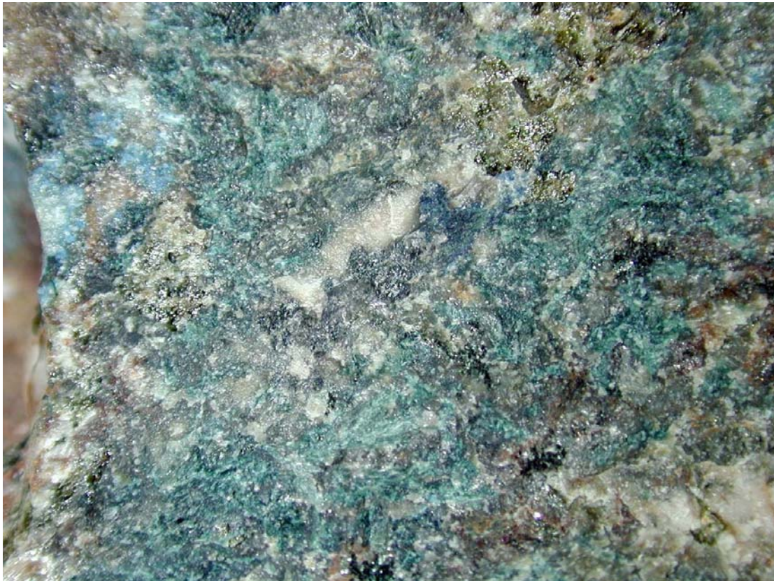
Figure 63: Gormanite-souzalite (bluish green) and associated minerals montebrasite (white) and scorzalite-lazulite (blue) from the Palermo #2 pegmatite. Field of view is approximately 2 cm.
