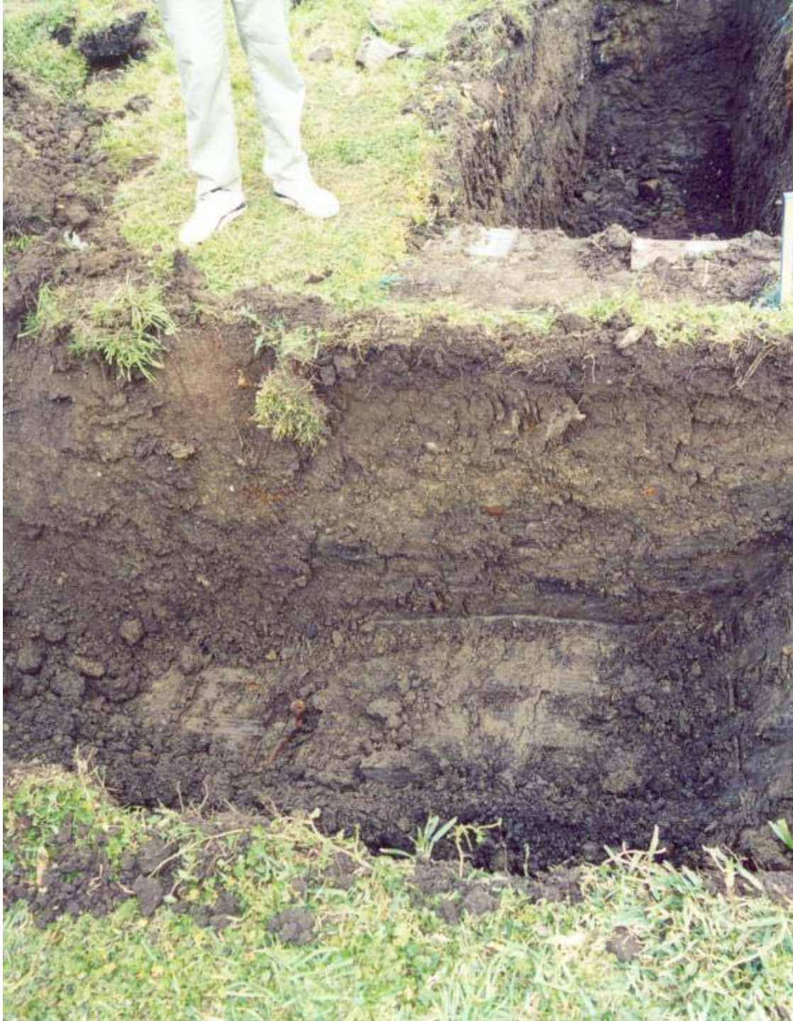
Figure 7: Excavated location flagged by TIR imaging. Grave identified at nearly 1 meter deep.
