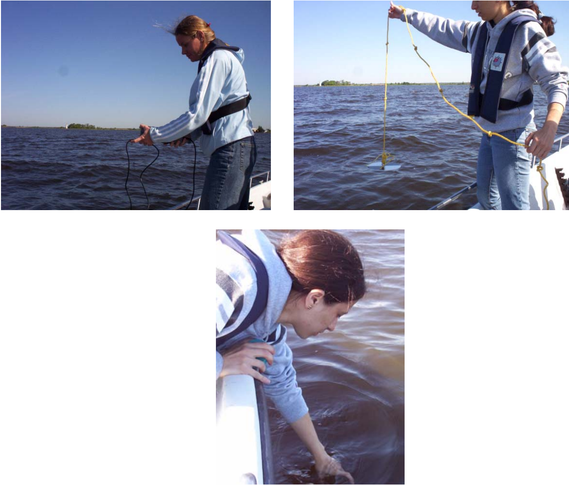
Figure 3.3: Sampling Collection and Field readings such as Secchi disk, DO, temperature and salinity
