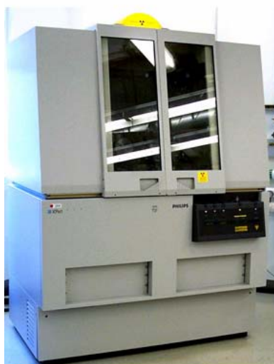
Figure 3.1: PW 3040/60 X'Pert Pro X-ray Diffraction System
