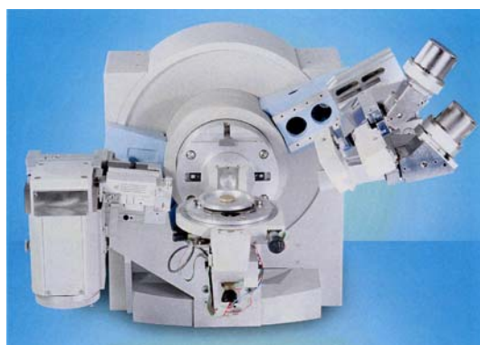
Figure 3.2 : Xpert PRO MPD(Multi Purpose Diffractometer) \theta - 2\theta system (from Xpert manual)
