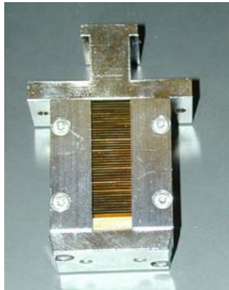
Figure 3.7: The 0.04 rad Soller slit (from Xpert manual)
