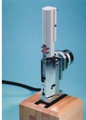
Figure 3.9: Programmable Receiving Slit with Fixed Anti Scatter Slit, Monochromator, Soller slit and detector (from Xpert manual)
