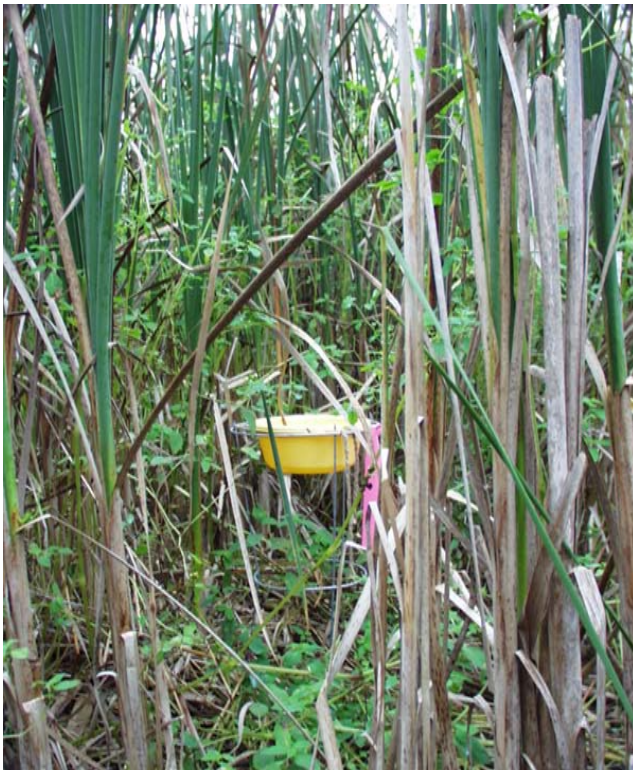
Figure 1. Yellow plastic pan trap suspended on wire tomato stand, within a Phragmites australis plot. The plastic bowl or pan is 20 cm diameter.
