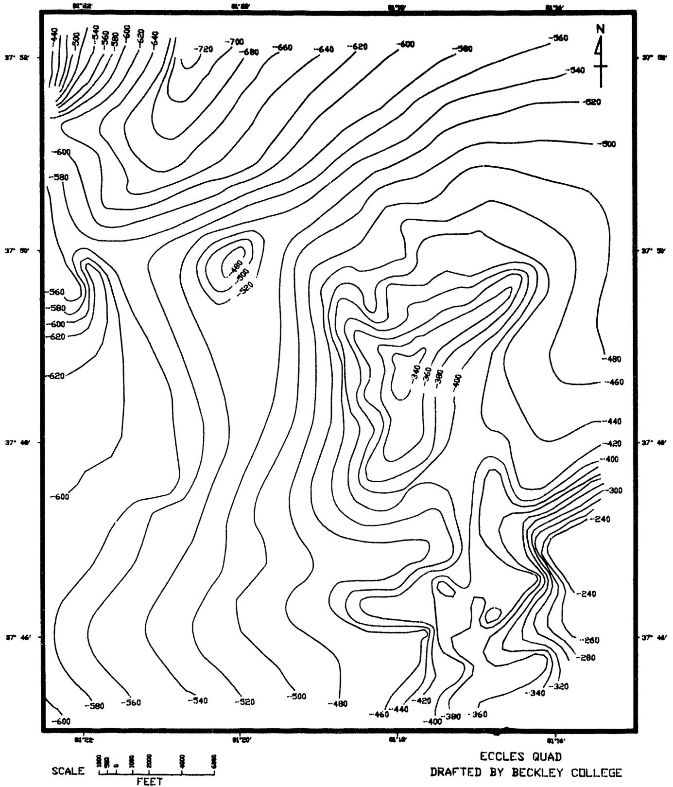
Figure 2.1.11 Structure on Top of the Big Lime, Eccles Quadrangle
