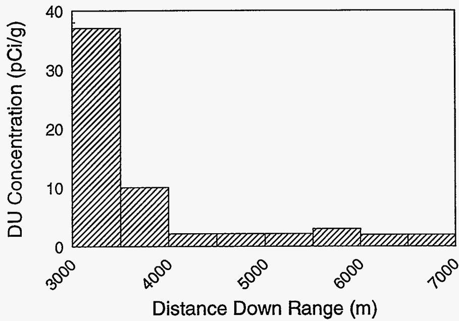
Figure 5. DU concentration in soils at GP 20. Data from grids north of the firing axis (Price, 1991).
