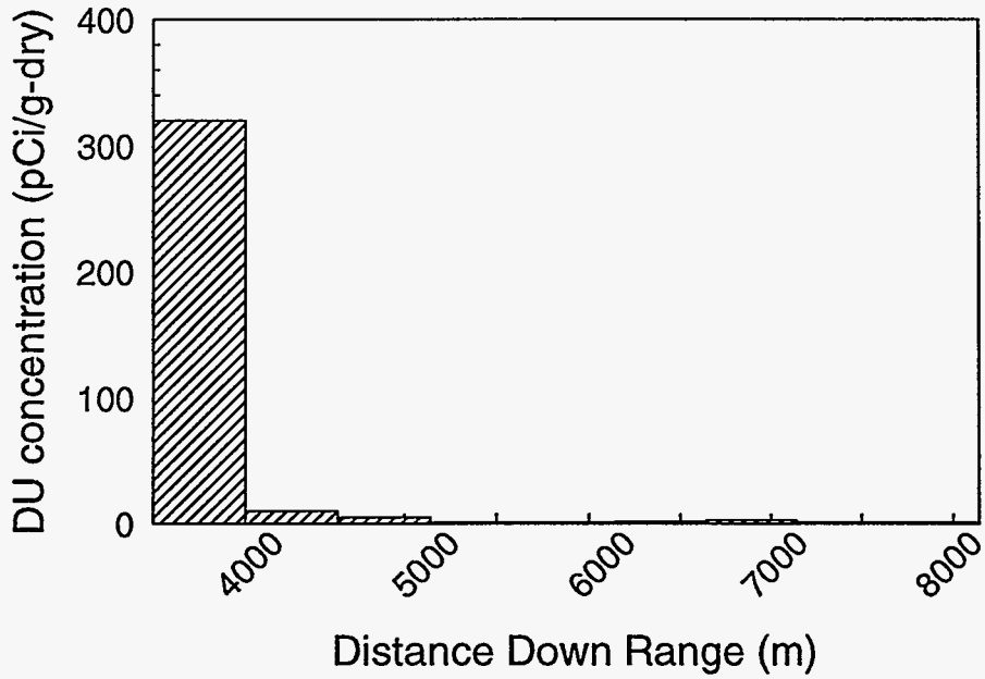
Figure 4. DU concentration in soils at GP 17A. Data from grids north of the firing axis (Price, 1991).
