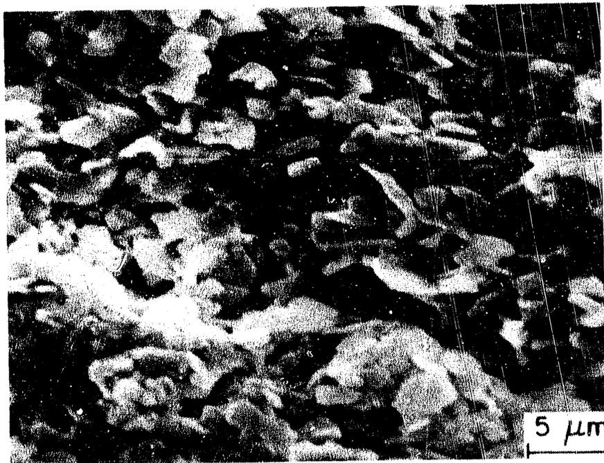
Fig. 13. SEM micrographs of boron nitride specimen after exposure at 1000°F in potassium liquid
