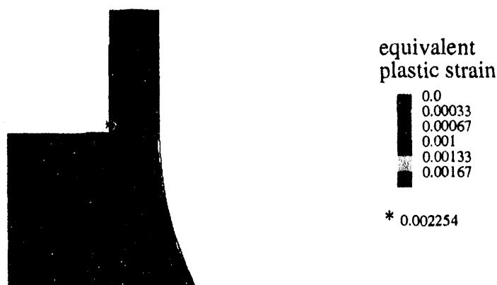
Figure 20. Equivalent plastic strain in the inner shell of inelastic truck cask
