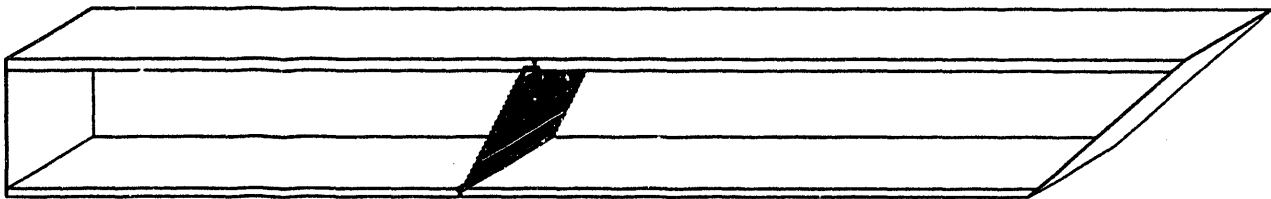
Figure 4C-4. The design chosen for the structural support of the barrel EMC modules. The mechanical structure utilizes back plates of 30-mm stainless steel and a 20-mm-thick aluminum front plate. Type 304 stainless steel end plates 3-mm thick and a 6-mm-thick stainless steel bulkhead at \eta \sim 0.5 provide additional support. The lead absorber sheets (not shown) are half the full module length and are captured by fixtures at the ends and middle of the module.
