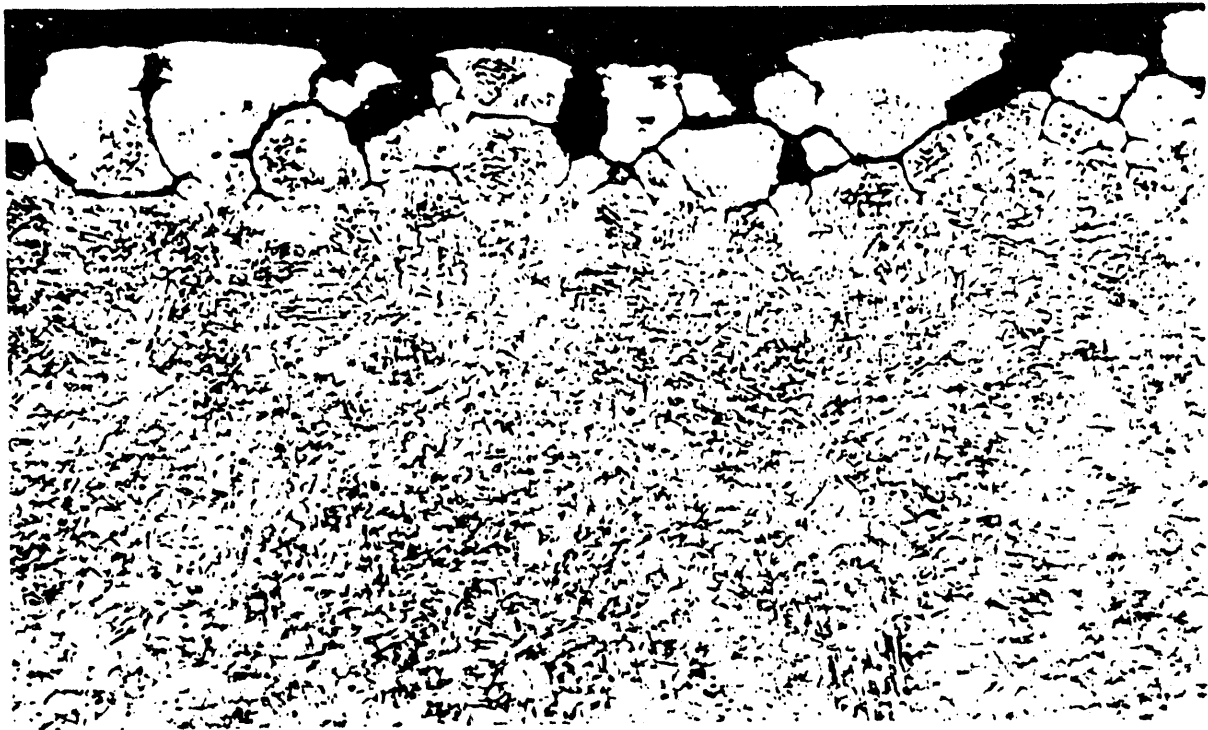
FIGURE 13 - Corroded surface of RA85H specimen coated with ash containing 10 wt% alkali sulfates after exposure for 800 hours at 700°C (1292°F) to flue gas containing 1.0 vol% SO 2 . (Note intergranular attack on specimen surface.)
