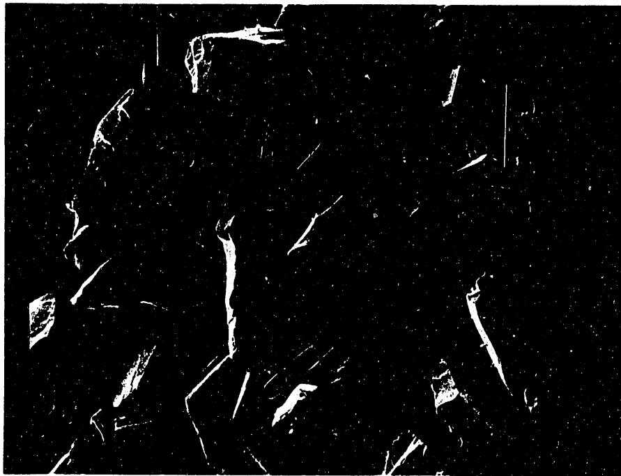
Figure 3. Scanning electron microscopy of 143 \mu\text{m} diameter SiC erodent: 3A—as received and 3B—after impacting a \text{Si}_3\text{N}_4 specimen at 100 m/s at normal incidence. The marker is 100 \mu\text{m} .
