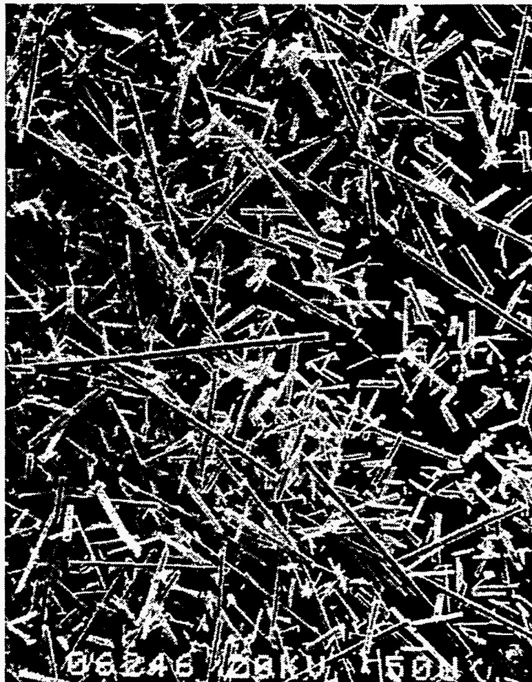
Figure 3.2.3-12 Typical graphite fiber appearance after ball milling for one hour.
