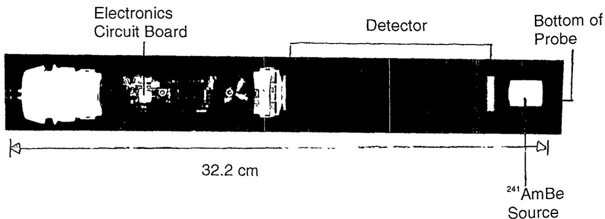
Fig. 9. X-ray of probe in Campbell Pacific moisture gauge (42% reduction of full-size image) showing locations of detector and <sup>241</sup>Am/Be source.
