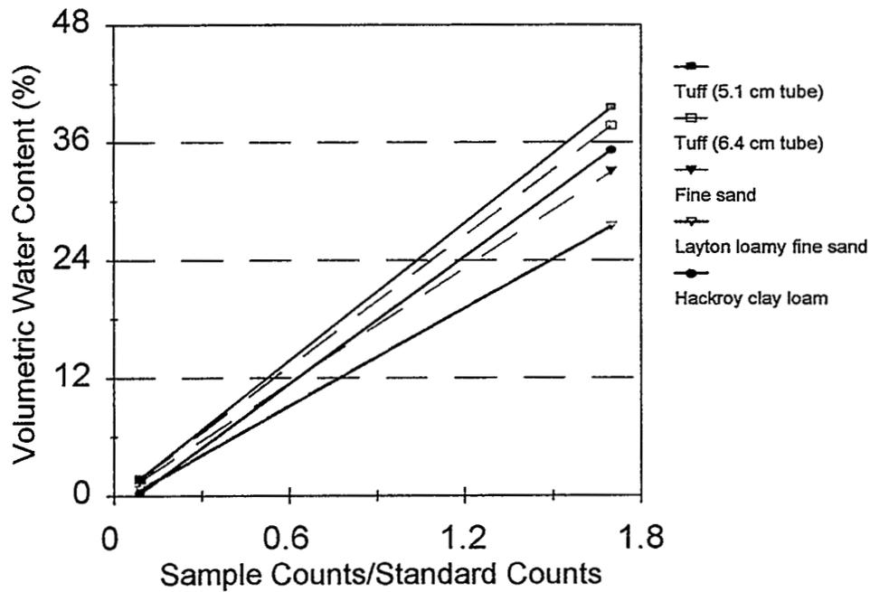
Fig. 46. Summary of regression predictions for all soil samples for neutron moisture gauges with serial numbers 5079 and 7832.
