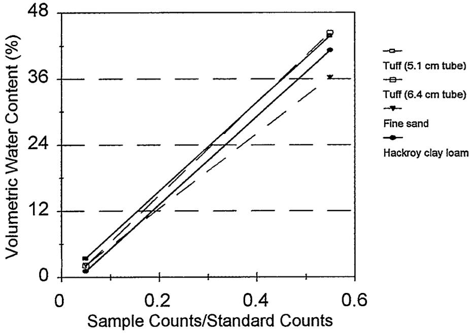
Fig. 47. Summary of regression predictions for all soil samples for neutron moisture gauge with serial number 5254.
