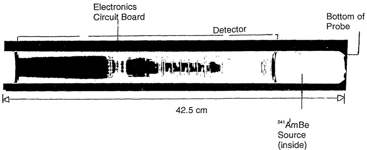
Fig. 11. X-ray of the terminal 42.5 cm of the 147-cm-long probe of the Gearhart-Owen moisture gauge (42% reduction of full size image) showing locations of detector and <sup>241</sup>Am/Be source.
