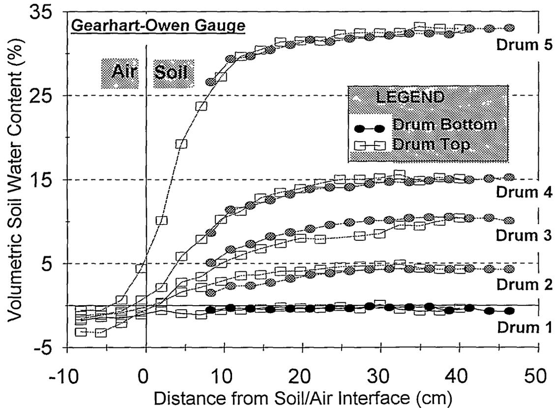
Fig. 17. Estimates of soil water content as a function of distance from the soil-air interface to the midpoint of the probe-sensitive area using the Gearhart-Owen moisture gauge. Calibration drums 1, 2, 3, 4, and 5 contained crushed tuff at average volumetric water contents of 0.12, 4.3, 8.6, 14.9, and 33%, respectively.
