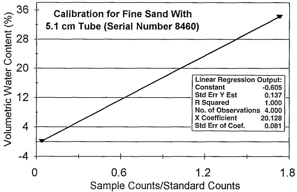
Fig. 41. Statistical analysis results for fine sand samples for neutron moisture gauges with serial numbers 8459 and 8460.
