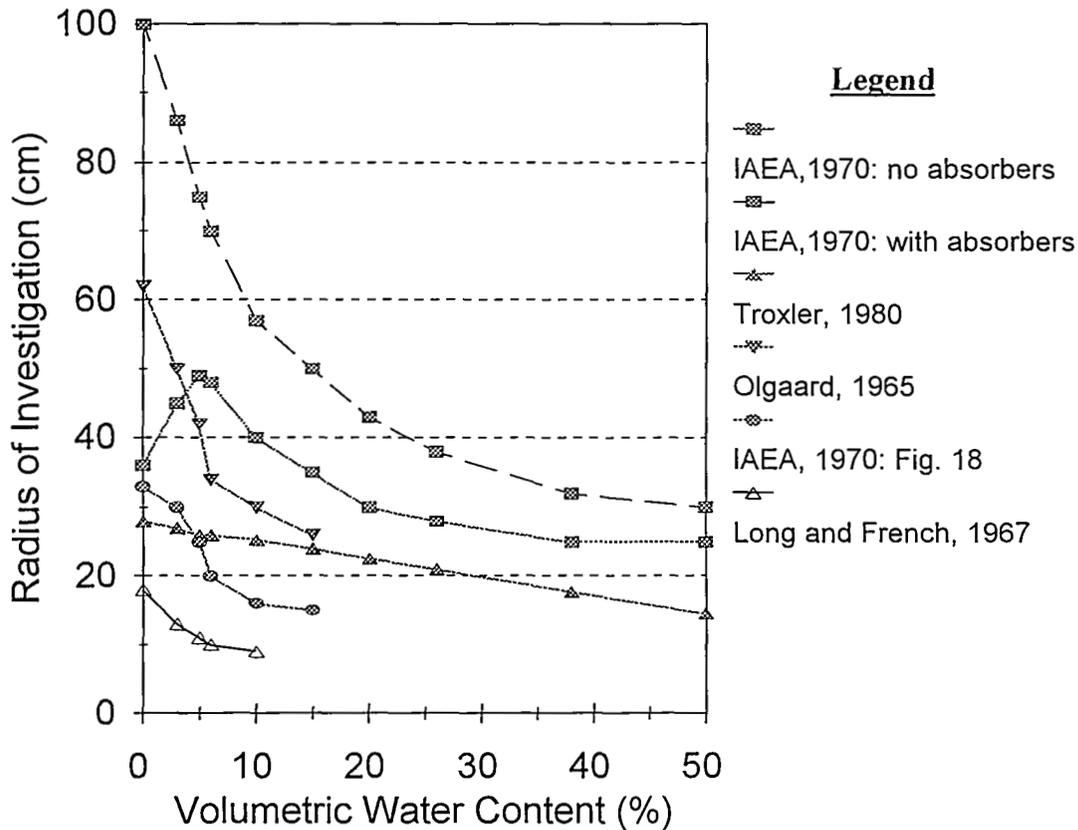
Fig. 1. Previous studies of  $R_j$  determinations and model predictions for neutron moisture gauges.
