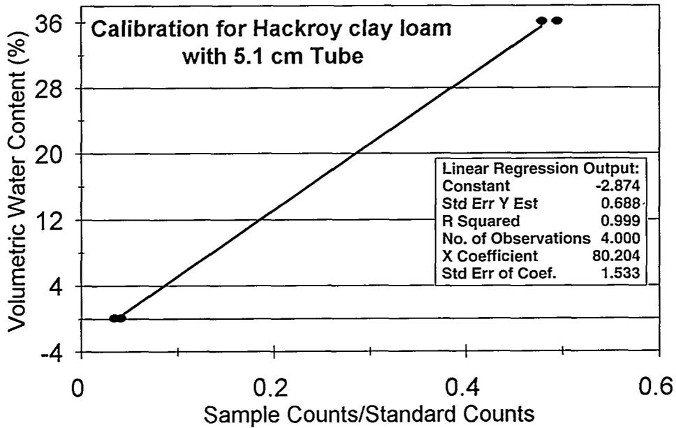
Fig. 38. Statistical analysis results for fine sand and Hackroy clay loam samples for neutron moisture gauge with serial number 5254.
