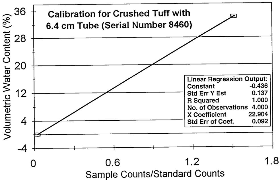
Fig. 40. Statistical analysis results for crushed tuff samples for neutron moisture gauges with serial numbers 8459 and 8460.
