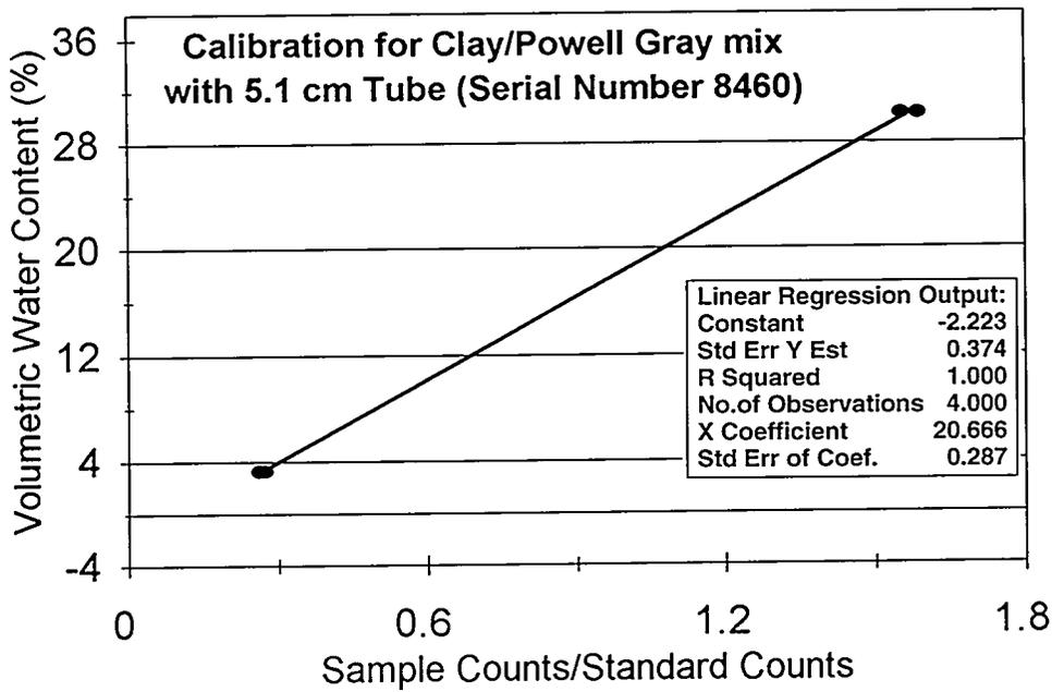
Fig. 44. Statistical analysis results for Bentonite/Powell Gray mixture samples for neutron moisture gauges with serial numbers 8459 and 8460.
