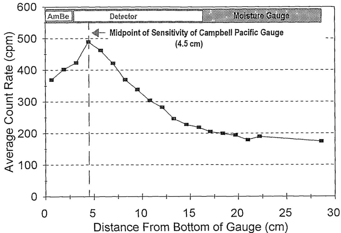
Fig. 12. Midpoint of sensitivity determination for the Campbell Pacific moisture gauge. The relationship of the midpoint of sensitivity to the gauge's  $^{241}\text{Am}/\text{Be}$  source and detector locations is also shown.
