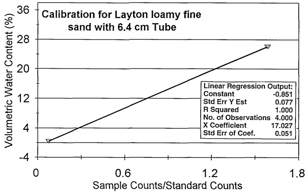
Fig. 33. Statistical analysis results for Layton loamy fine sample for neutron moisture gauge with serial number 5079.
