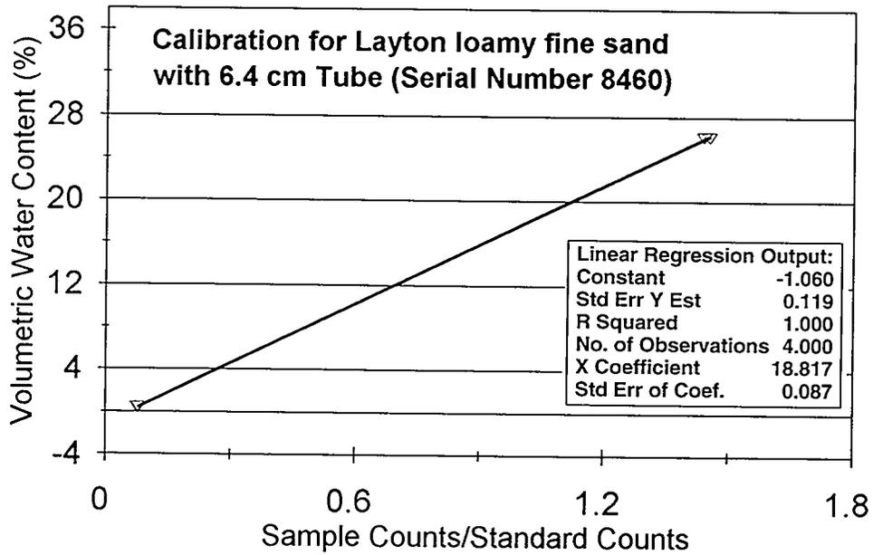
Fig. 43. Statistical analysis results for Layton loamy fine sand samples for neutron moisture gauges with serial numbers 8459 and 8460.
