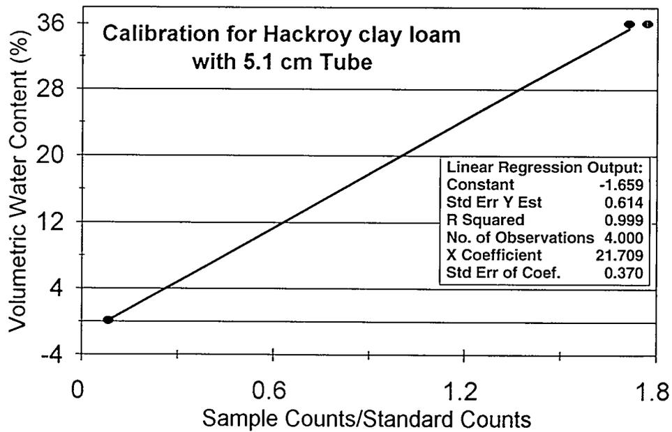
Fig. 35. Statistical analysis results for fine sand and Hackroy clay loam samples for neutron moisture gauge with serial number 7832.
