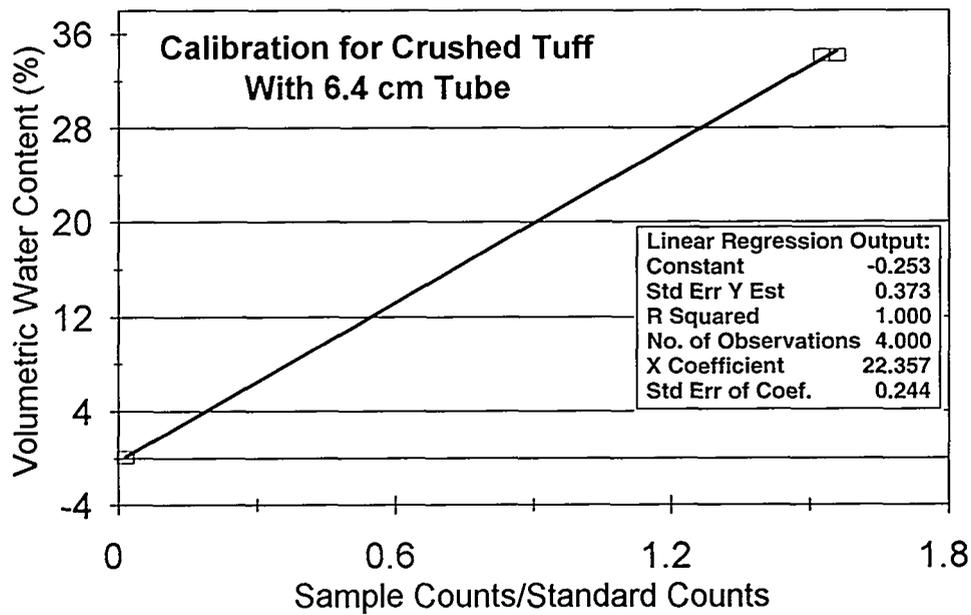
Fig. 34. Statistical analysis results for crushed tuff samples for neutron moisture gauge with serial number 7832.
