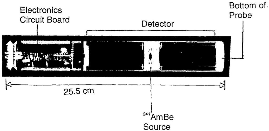
Fig. 10. X-ray of probe in Troxler moisture gauge (42% reduction of full size image) showing locations of detector and <sup>241</sup>Am/Be source.
