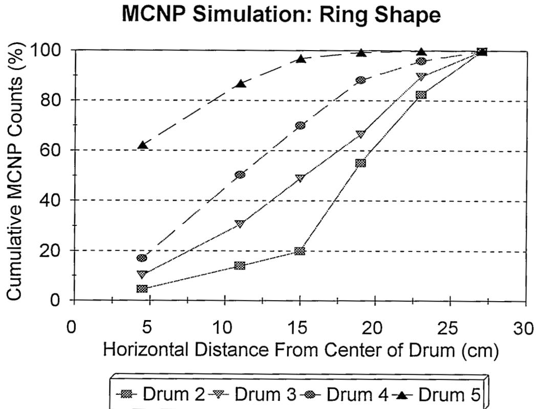
Fig. 20. MCNP modeling results for simulations of crushed tuff in calibration drums with MCNP cells consisting of concentric rings. Calibration drums 2, 3, 4, and 5 contained crushed tuff at average volumetric water contents of 4.3, 8.6, 14.9, and 33%, respectively.
