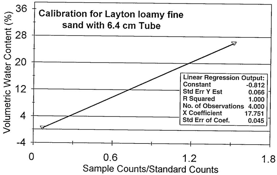
Fig. 27. Statistical analysis results for Layton loamy fine sand sample for neutron moisture gauge with serial number 4274.
