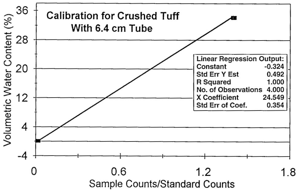
Fig. 25. Statistical analysis results for crushed tuff samples for neutron moisture gauge with serial number 4274.
