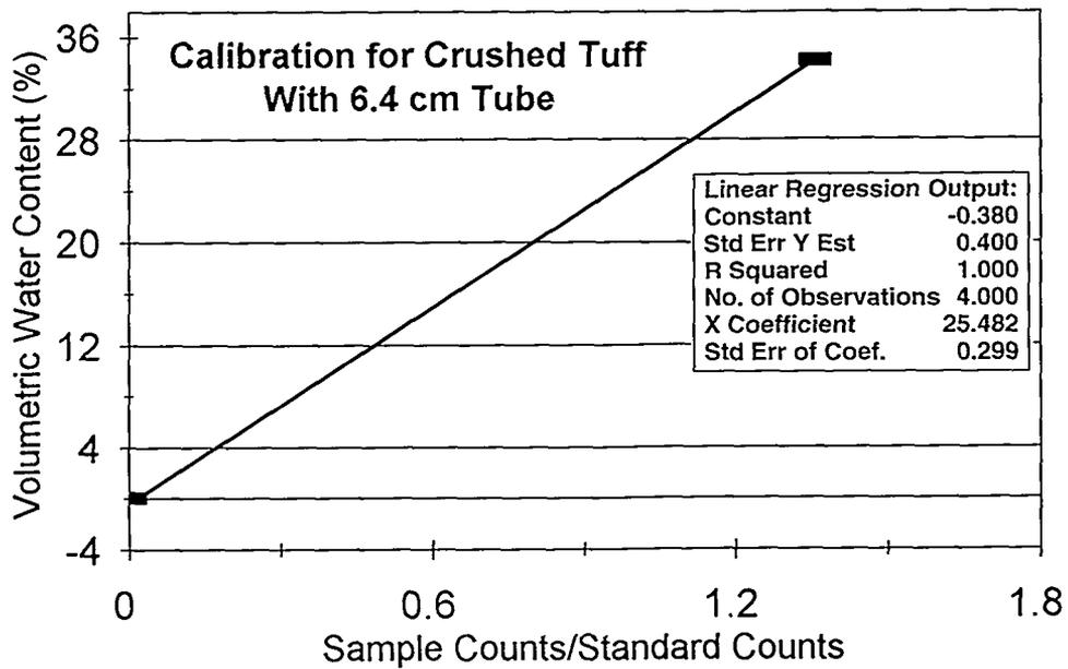
Fig. 28. Statistical analysis results for crushed tuff samples for neutron moisture gauge with serial number 4519.
