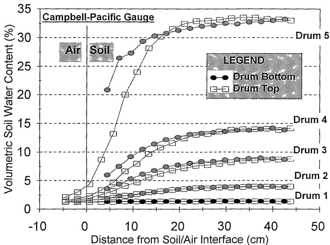
Fig. 15. Estimates of soil water content as a function of distance from the soil-air interface to the midpoint of the probe-sensitive area using the Campbell Pacific moisture gauge. Calibration drums 1, 2, 3, 4, and 5 contained crushed tuff at average volumetric water contents of 0.12, 4.3, 8.6, 14.9 and 33%, respectively.
