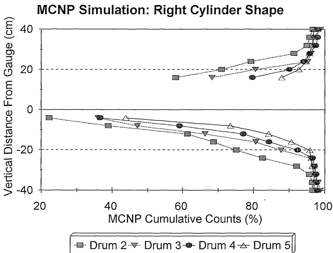
Fig. 21. MCNP modeling results for simulations of crushed tuff in calibration drums with MCNP cells consisting of a stack of many right cylindrical segments. Calibration drums 2, 3, 4, and 5 contained crushed tuff at average volumetric water contents of 4.3, 8.6, 14.9, and 33%, respectively.
