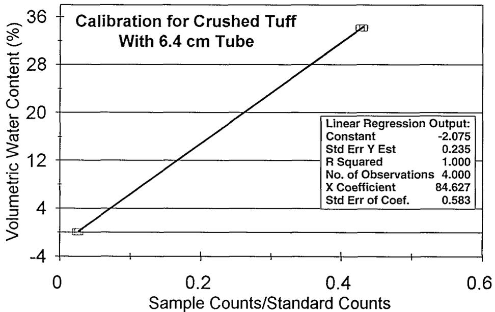
Fig. 37. Statistical analysis results for crushed tuff samples for neutron moisture gauge with serial number 5254.
