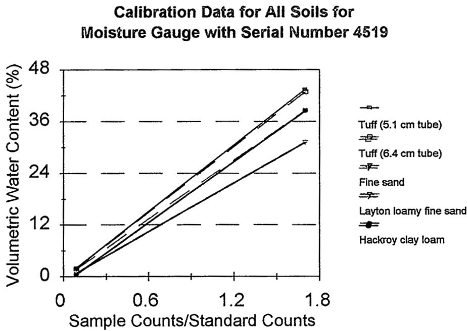
Fig. 45. Summary of regression predictions for all soil samples for neutron moisture gauges with serial numbers 4274 and 4519.
