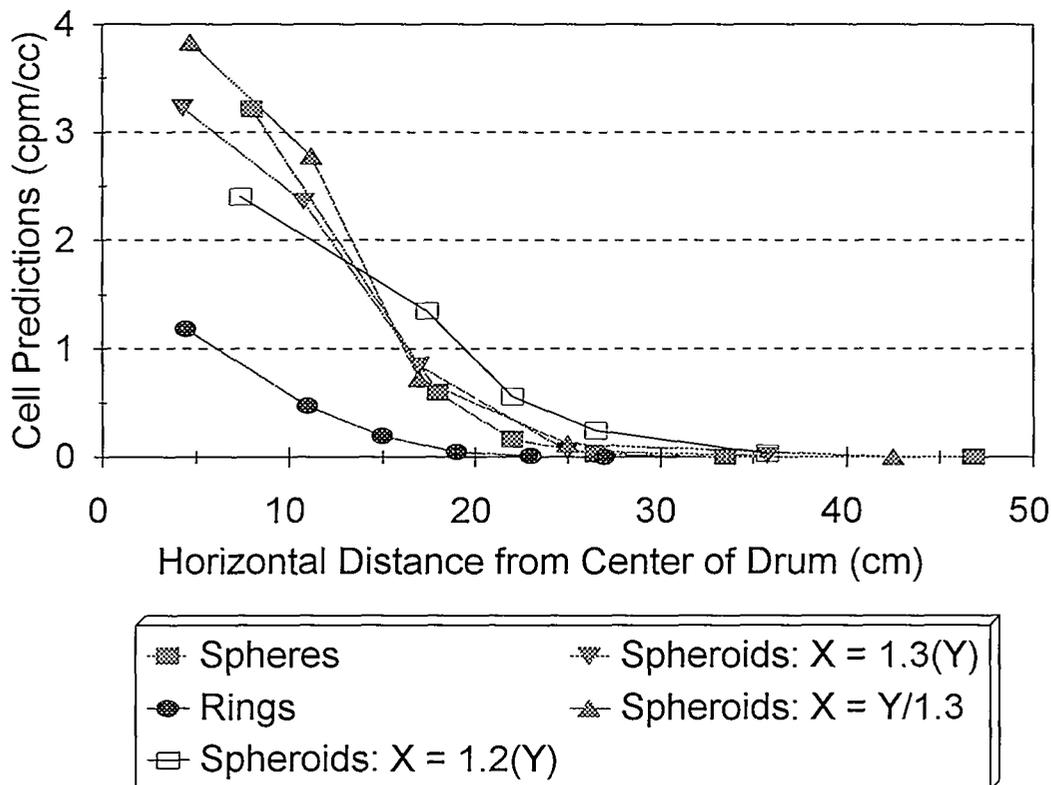
Fig. 24. MCNP shape simulations for calibration drum 5 containing crushed tuff at an average volumetric water content of 33%.
