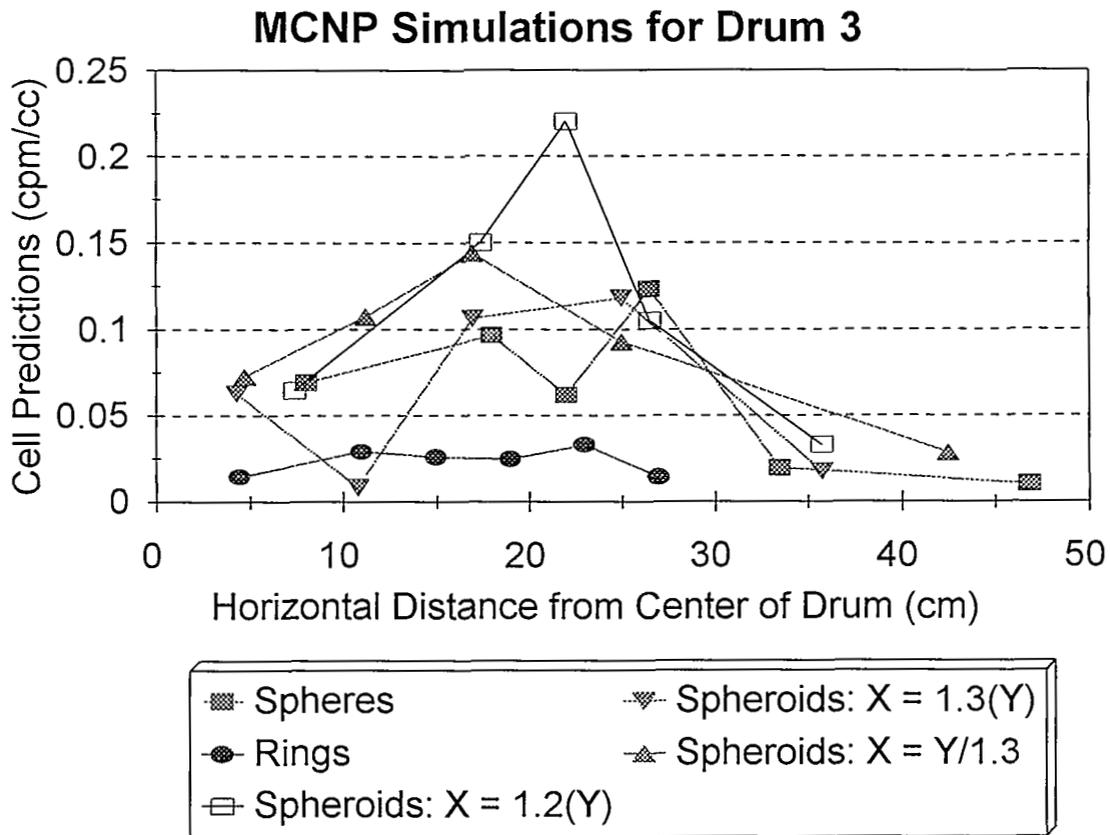
Fig. 22. MCNP shape simulations for calibration drum 3 containing crushed tuff at an average volumetric water content of 8.6%.
