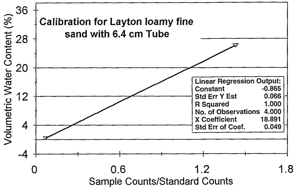
Fig. 30. Statistical analysis results for Layton loamy fine sand sample for neutron moisture gauge with serial number 4519.
