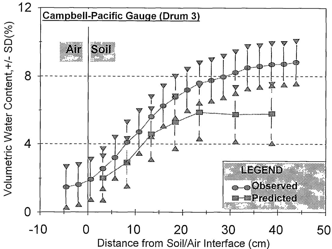
Fig. 19. Observed measurements and MCNP model predictions of volumetric crushed-tuff water content near the soil-air interface of calibration drum 3 containing tuff at an average volumetric water content of 8.6%.
