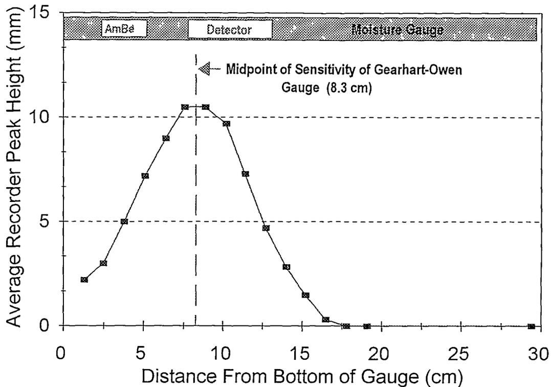
Fig. 14. Midpoint of sensitivity determination for the Gearhart-Owen moisture gauge. The relationship of the midpoint of sensitivity to the gauge's  $^{241}\text{Am}/\text{Be}$  source and detector locations is also shown.
