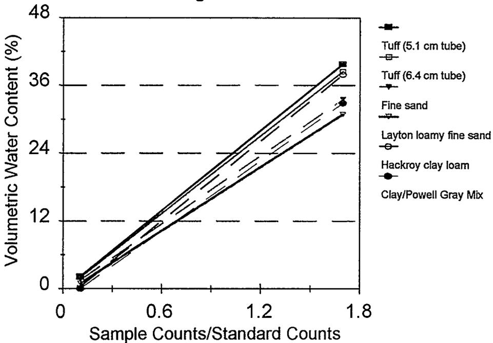
Fig. 48. Summary of regression predictions for all soil samples for neutron moisture gauges with serial numbers 8459 and 8460.
