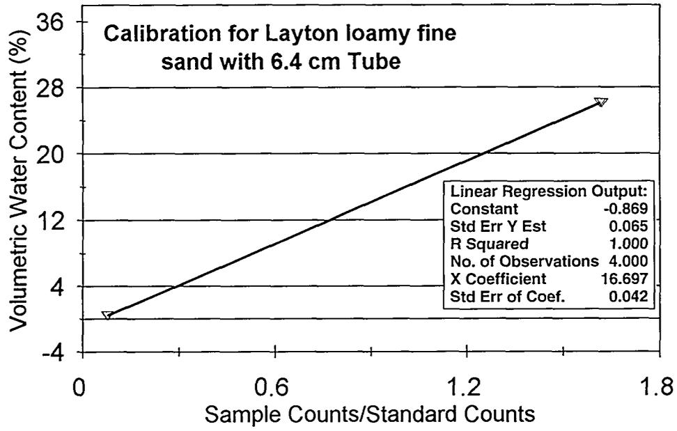
Fig. 36. Statistical analysis results for Layton loamy fine sand samples for neutron moisture gauge with serial number 7832.
