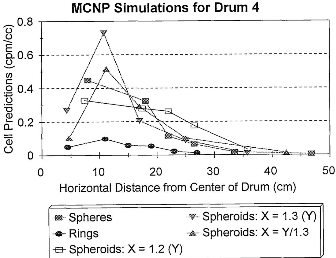
Fig. 23. MCNP shape simulations for calibration drum 4 containing crushed tuff at an average volumetric water content of 14.9%.
