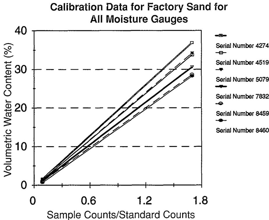
Fig. 49. Summary of regression predictions for the standard factory sand samples for all neutron moisture gauges.
