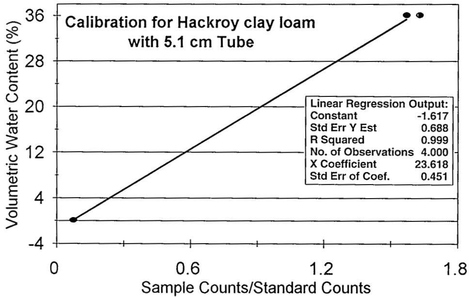
Fig. 29. Statistical analysis results for fine sand and Hackroy clay loam samples for neutron moisture gauge with serial number 4519.
