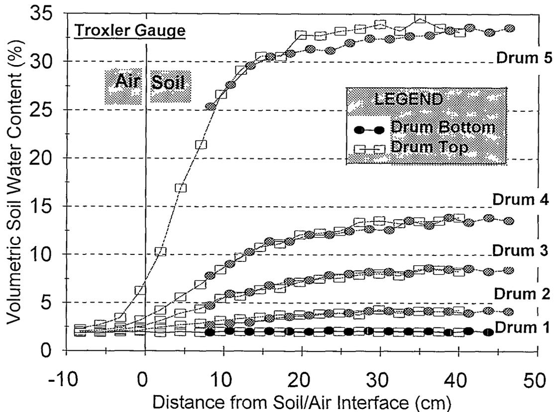
Fig. 16. Estimates of soil water content as a function of distance from the soil-air interface to the midpoint of the probe-sensitive area using the Troxler moisture gauge. Calibration drums 1, 2, 3, 4, and 5 contained crushed tuff at average volumetric water contents of 0.12, 4.3, 8.6, 14.9, and 33%, respectively.
