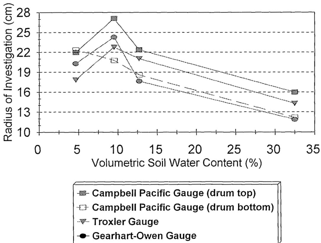
Fig. 18. Rj determinations as a function of crushed-tuff water content for the three moisture gauges used in the study.
