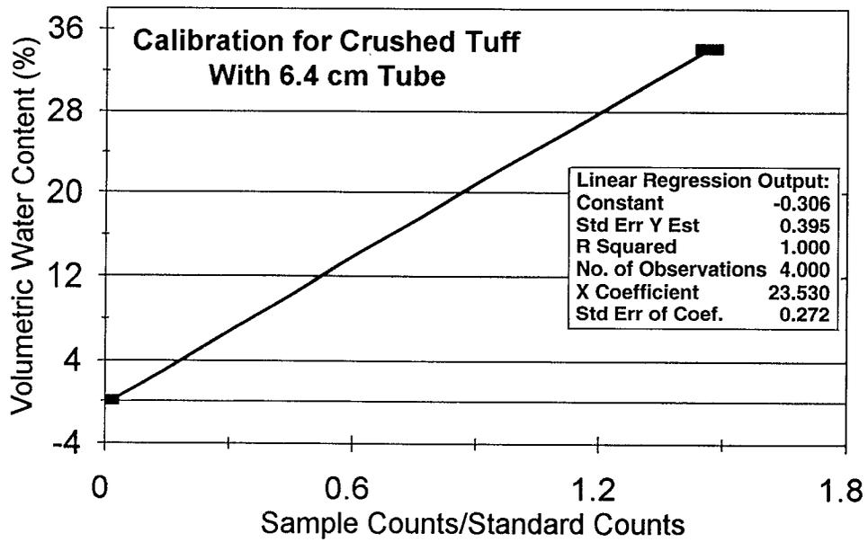
Fig. 31. Statistical analysis results for crushed tuff samples for neutron moisture gauge with serial number 5079.
