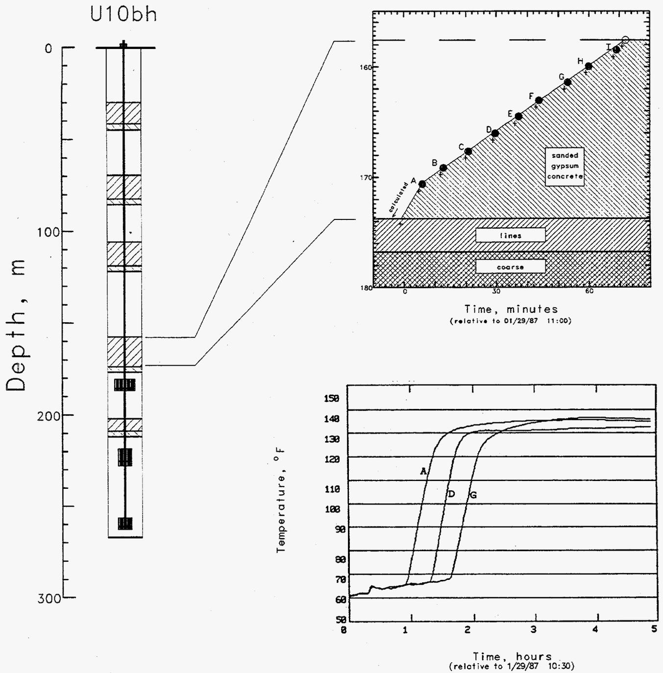
Figure 2.2 Sanded gypsum emplacement for plug #2. The upper and lower plug boundaries were calculated or determined with a tag line (open circle). Solid symbols indicate the probe elevations. Probes labeled A, D, and G included temperature sensors.
