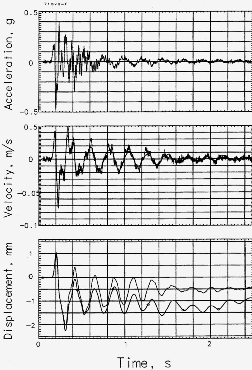
Figure 4.1 Explosion-induced vertical motion of the recording trailer (station 71). Records annotated with an 'a' are derived from the accelerometer.
