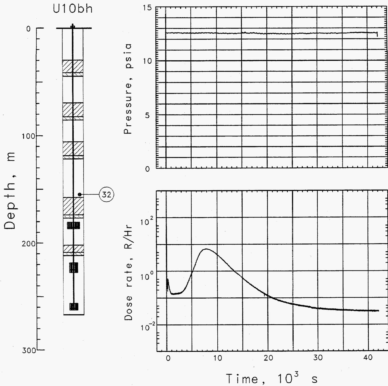
Figure 3.2 Pressure and radiation measured in the course stemming above SGC plug #2 (station 32 at 152 m depth). First arrival of radiation is about 22 s.
