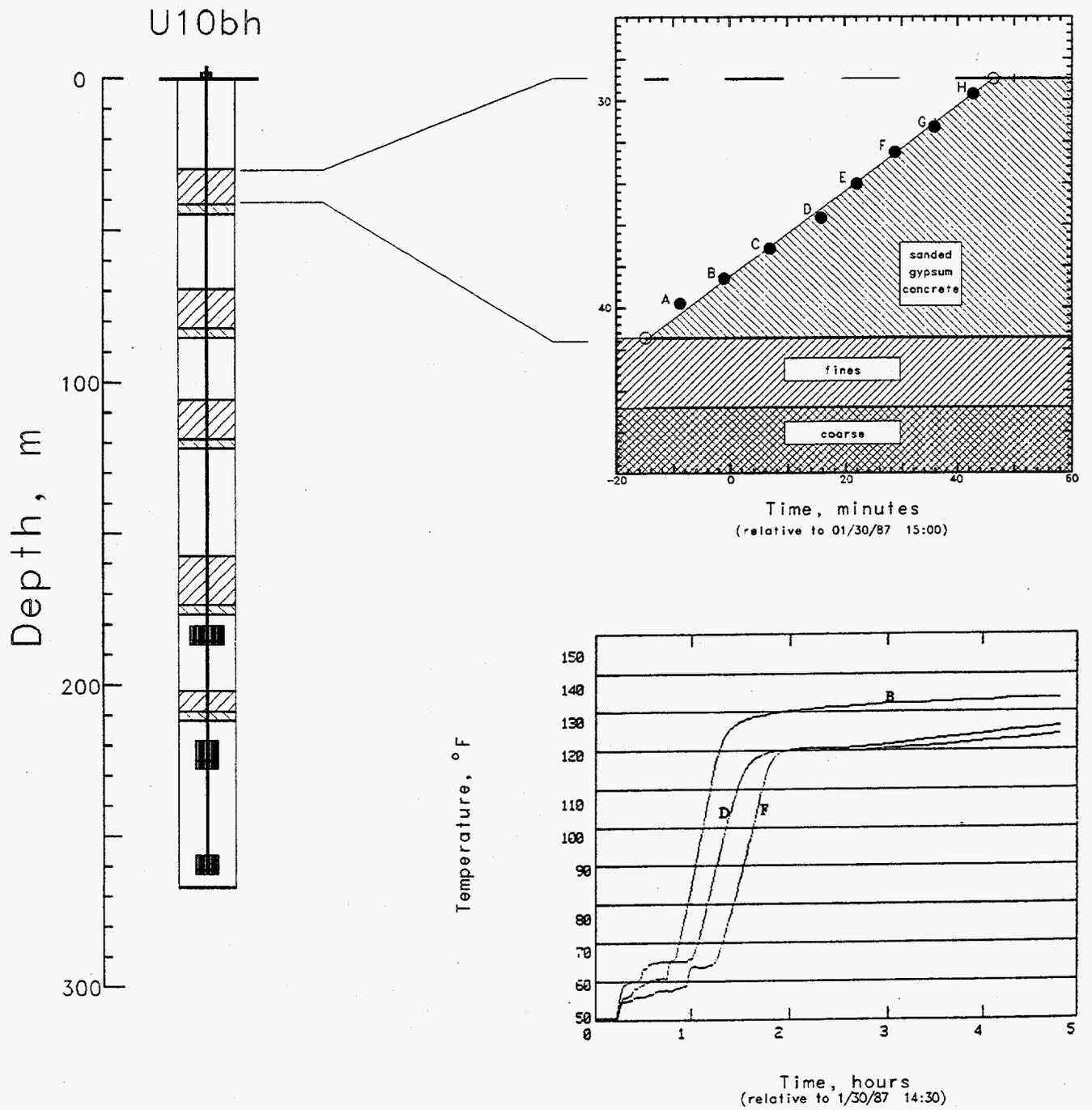
Figure 2.5 Sanded gypsum emplacement for plug #5. The upper and lower plug boundaries were determined with a tag line (open circles). Solid symbols indicate the probe elevations. Probes labeled B, D, and F included temperature sensors.
