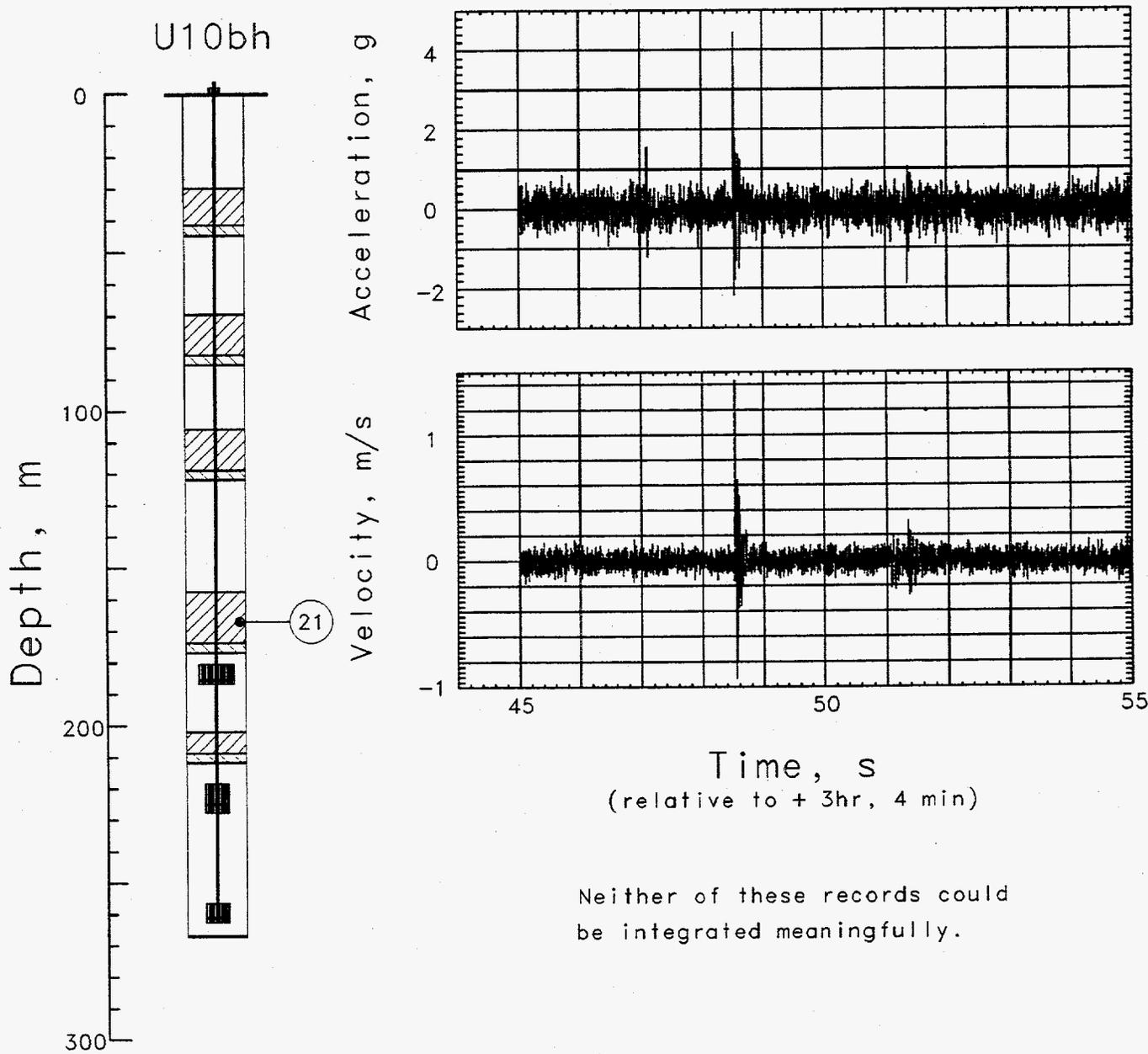
Figure 3.15 Possible collapse-induced signals in plug #2 at a depth of 166 m (station 21). No discernible displacement was detected.
