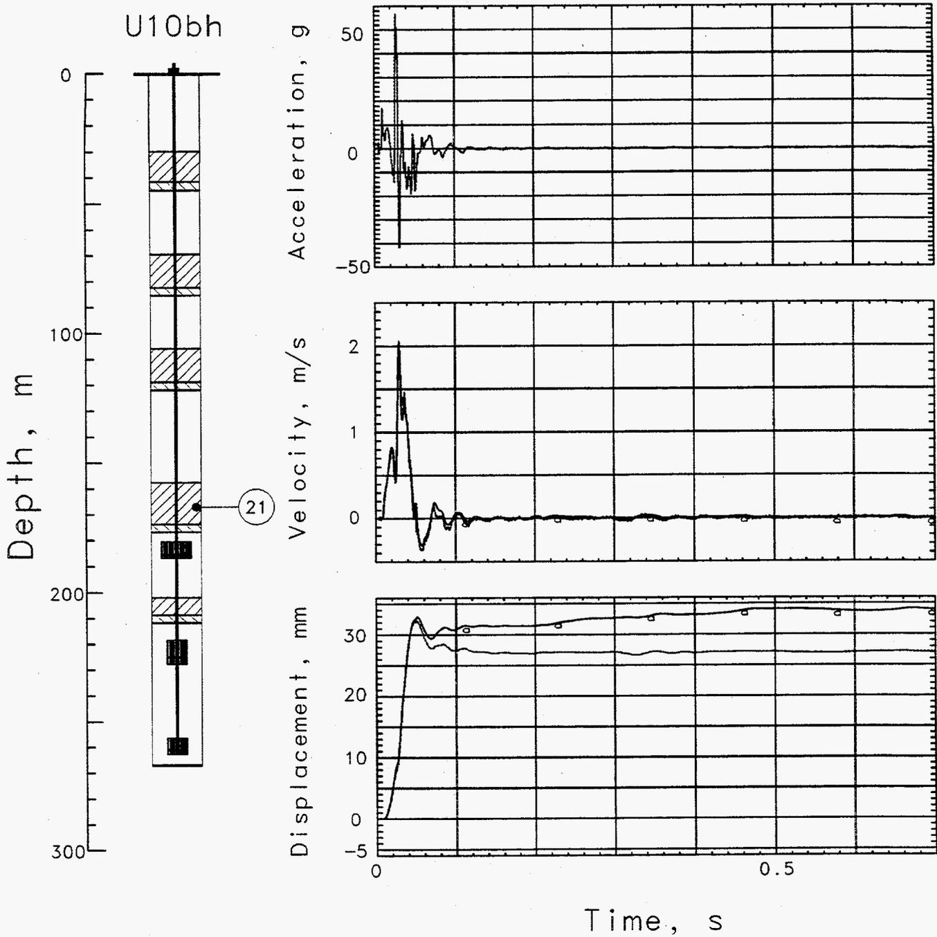
Figure 3.14 Explosion-induced vertical motion of plug #2 at a depth of 166 m (station 21). Records annotated with an 'a' are derived from the accelerometer.
