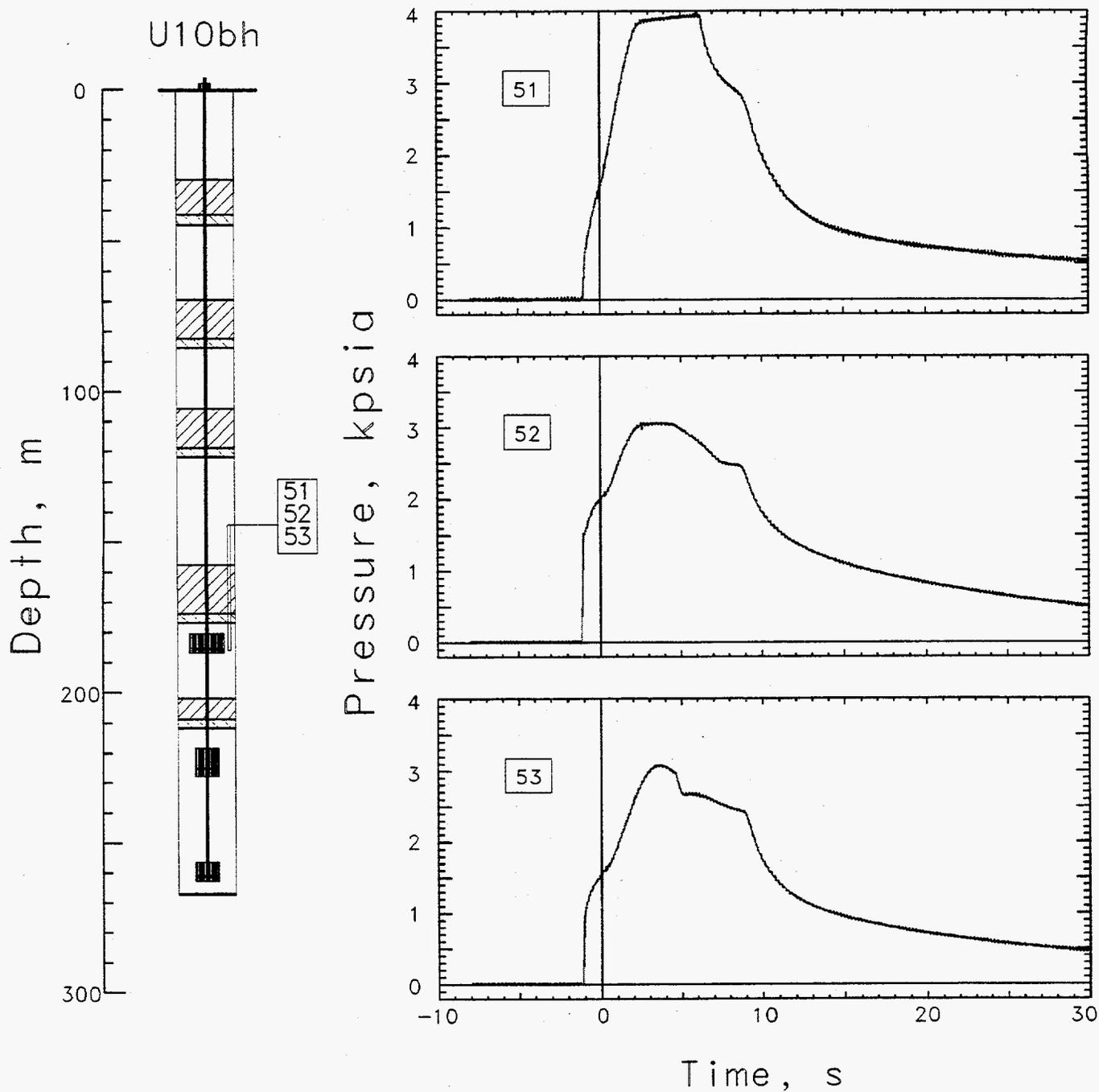
Figure 3.8 Early time wave forms of pressure measured through tubes extending from a depth of 145 m to near the W.P. A pressure of about 4000 psi from a 1.2 l reservoir of dry nitrogen was applied before shot time.
