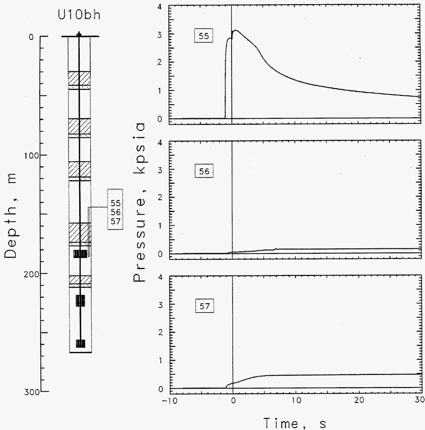
Figure 3.10 Early time wave forms of pressure measured through tubes extending from a depth of 145 m to near the W.P. A pressure of about 4000 psi from a 1.2 l reservoir of dry nitrogen was applied before shot time. These transducers were an extension of the gas sample system which extended upward to the radio chemistry trailer.
