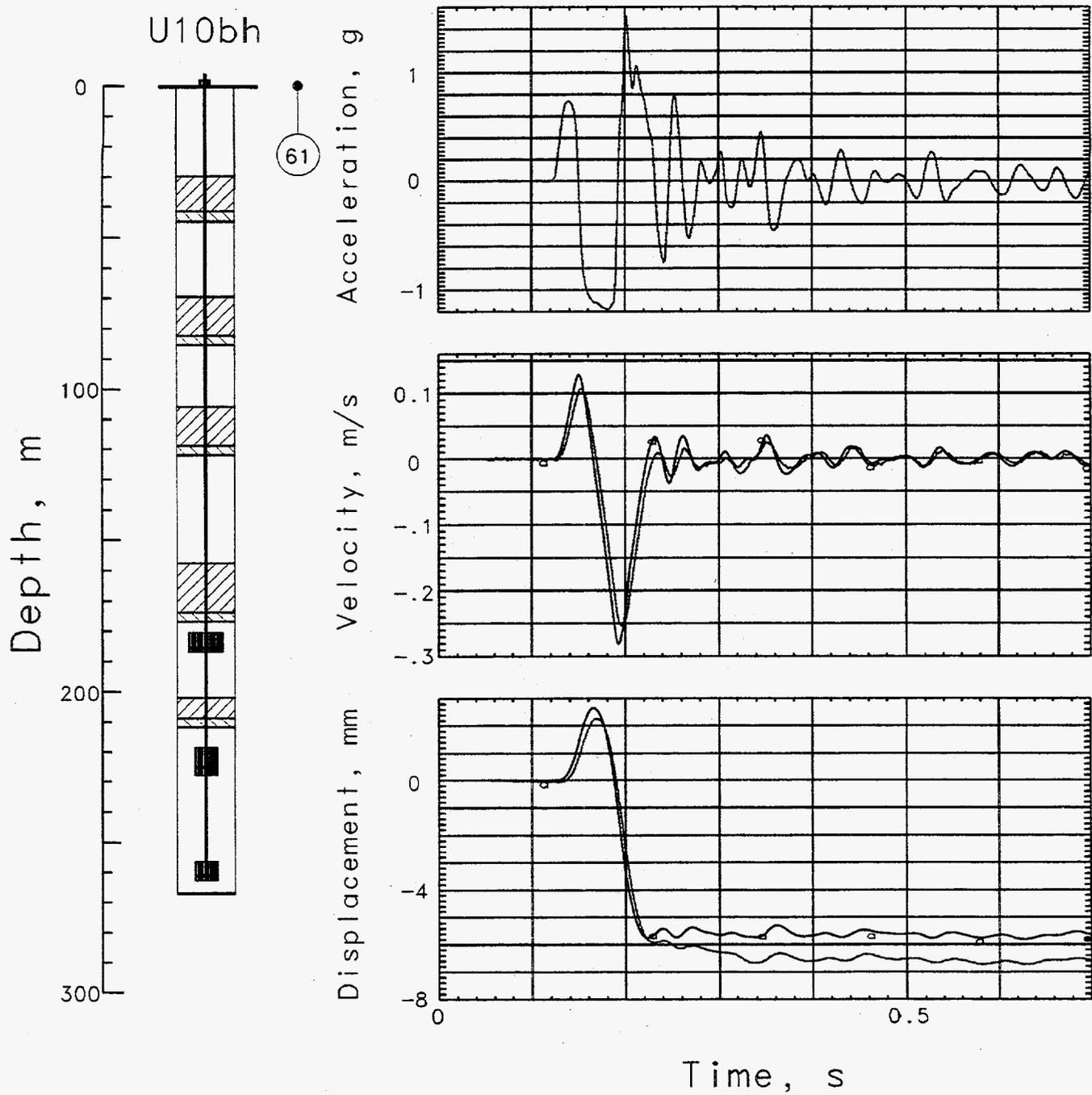
Figure 3.18 Explosion-induced vertical motion 0.91 m deep in the ground surface at a horizontal distance of 15.24 m from Surface Ground Zero (station 61). Records annotated with an 'a' are derived from the accelerometer.
