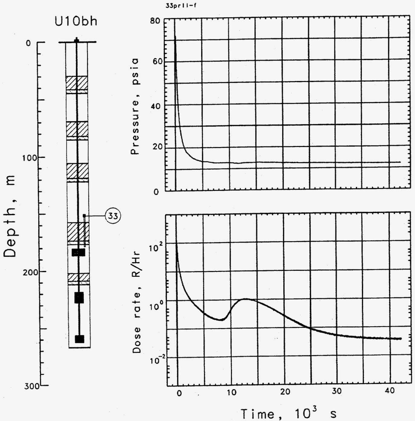
Figure 3.3 Pressure and radiation challenging the second plug as measured in the coarse stemming below it (station 33 at 148 m depth). Measurements were taken through a hose that penetrated the second plug and extended about 4 m below it to a depth of 178 m. First arrival of radiation is unknown, but probably before 25 s.
