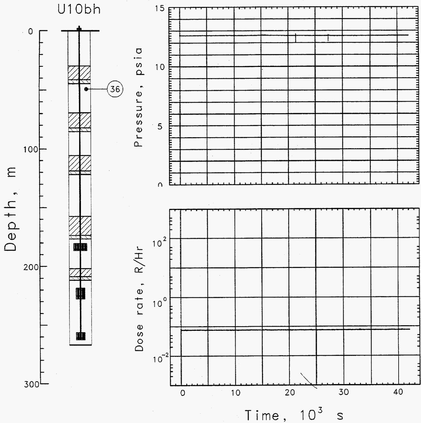
Figure 3.6 Pressure and radiation measured in the coarse stemming below SGC plug #5 (stations 36 at 45 m depth and 13 at 48 m depth).
