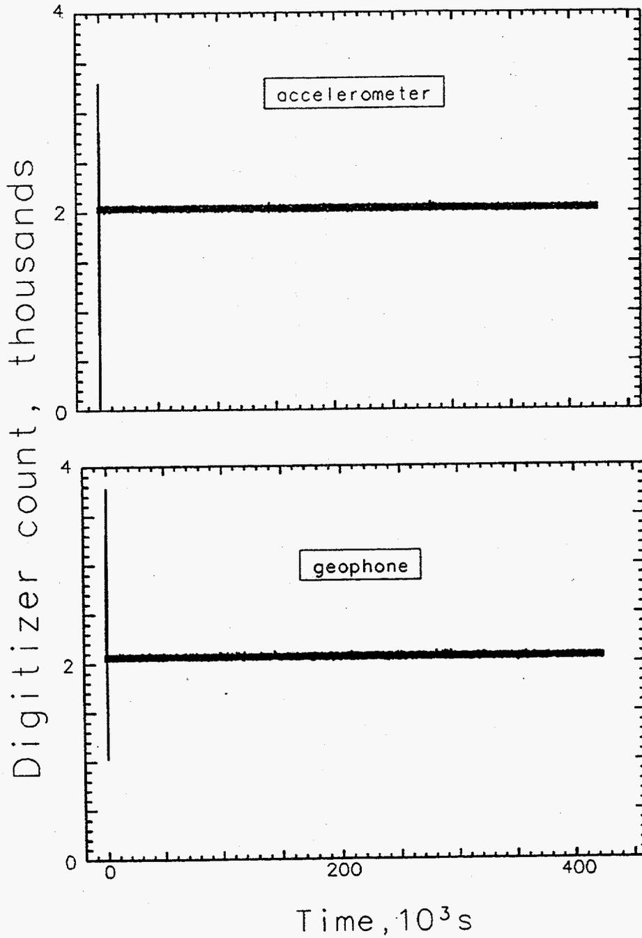
Figure 4.4 Data from the vertical geophone and sensitive accelerometer mounted in the ground surface at the recording trailer (station 63). Note that there is no detectable motion after the first explosion-induced shock.
