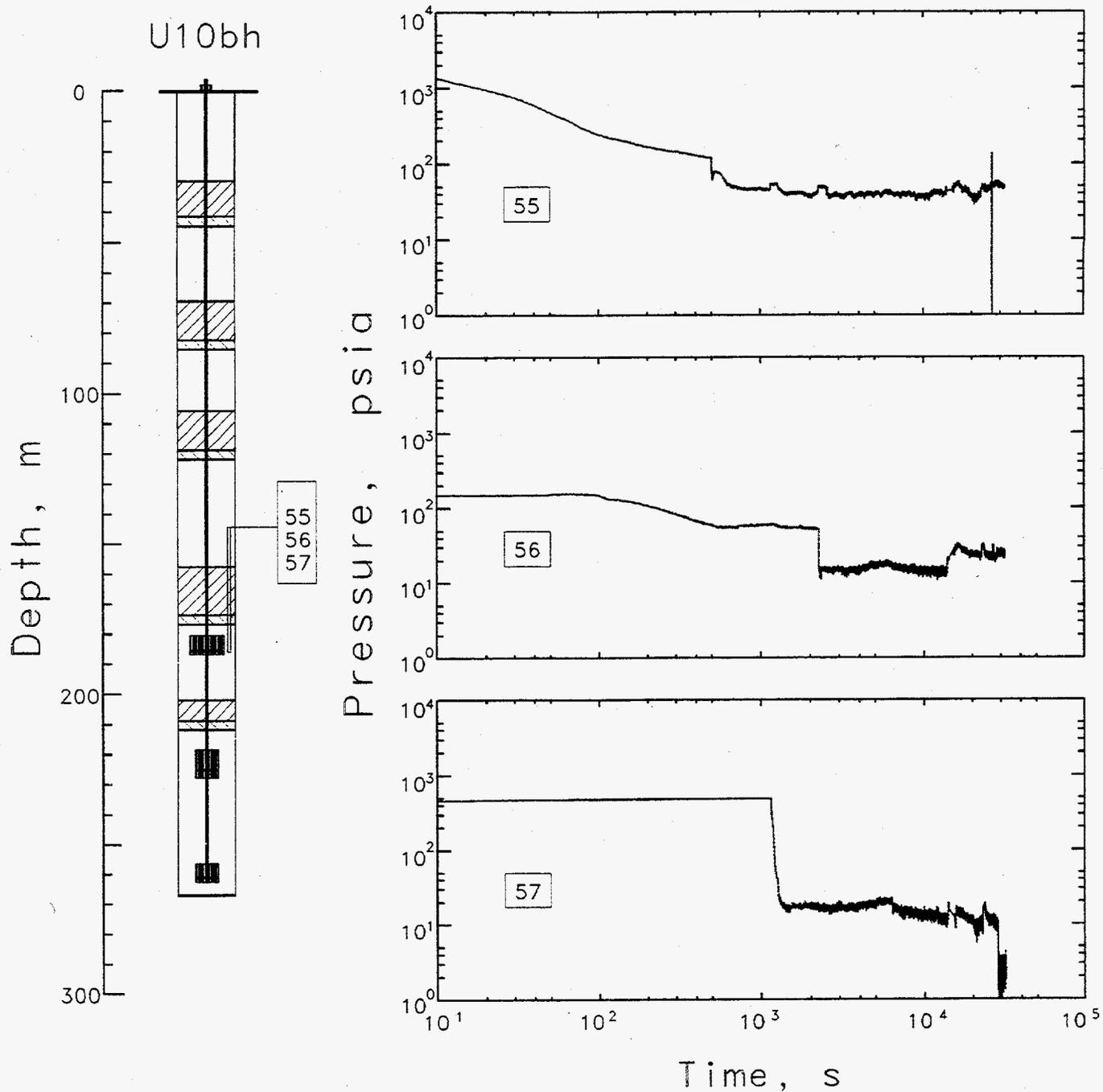
Figure 3.11 Late time wave forms of pressure measured through tubes extending from a depth of 145 m to near the W.P. A pressure of about 4000 psi from a 1.2 l reservoir of dry nitrogen was applied before shot time. These transducers were an extension of the gas sample system which extended upward to the radio chemistry trailer.
