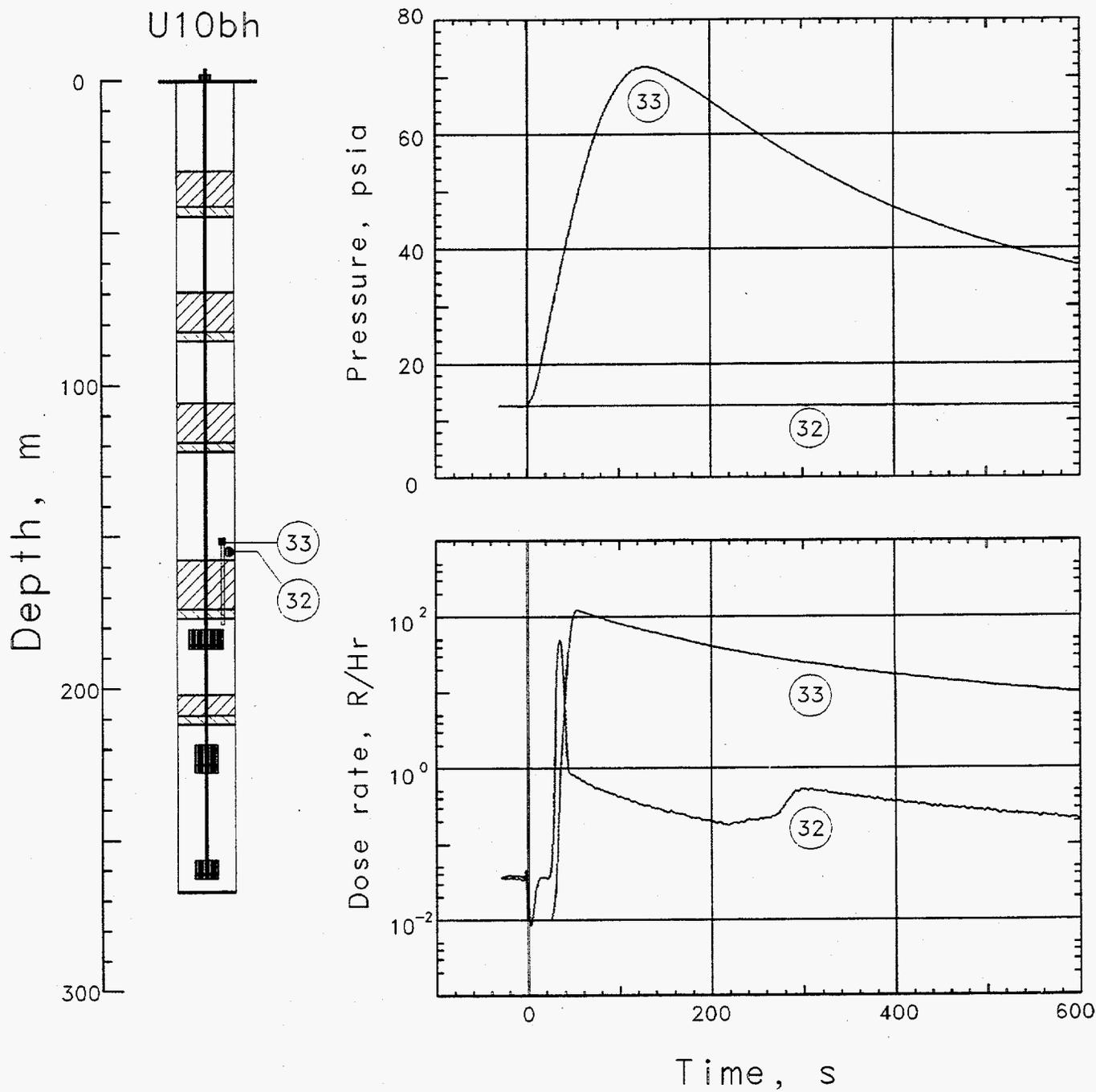
Figure 3.7 Comparison of pressures across the second plug and the radiation measured immediately above this plug. Pressure challenging the plug reached a peak of 60 psi at about 130 s. Radiation arrived at both stations at about 22 s.
