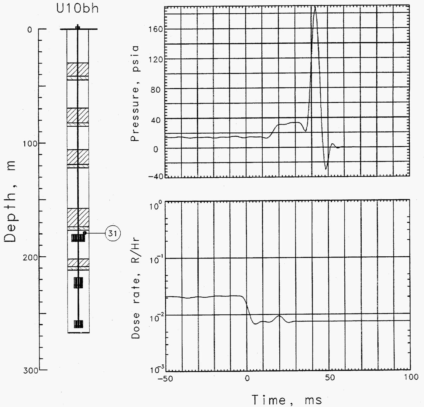
Figure 3.1 Pressure and radiation measured in the coarse stemming below SGC plug #2 (station 31 at 178 m depth). Station signals were lost shortly after detonation, presumably due to shock arrival.
