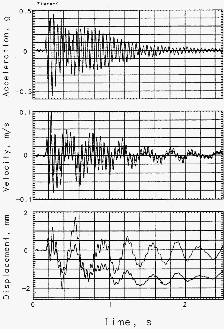
Figure 4.2 Explosion-induced horizontal-radial motion of the recording trailer (station 71). Records annotated with an 'a' are derived from the accelerometer.
