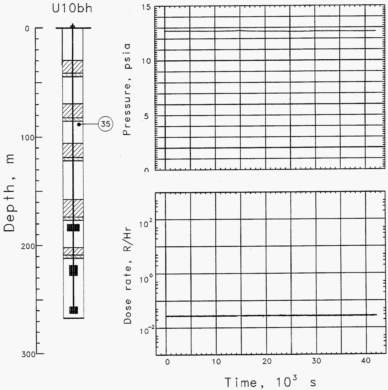
Figure 3.5 Pressure and radiation measured in the coarse stemming below SGC plug #4 (stations 35 at 85 m depth and 12 at 88 m depth).
