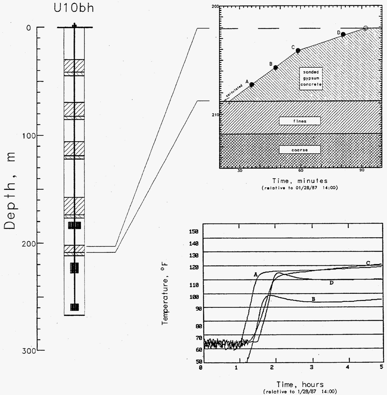
Figure 2.1 Sanded gypsum emplacement for plug #1. The upper and lower plug boundaries were calculated or determined with a tag line (open circle). Solid symbols indicate the probe elevations. All probes included temperature sensors.
