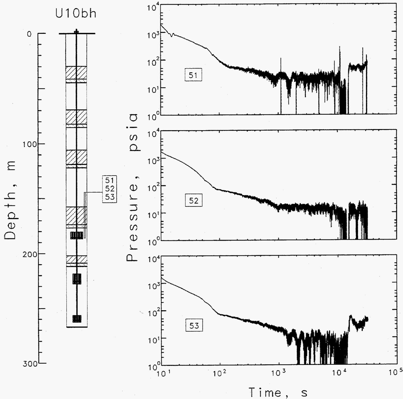
Figure 3.9 Late time wave forms of pressure measured through tubes extending from a depth of 145 m to near the W.P. A pressure of about 4000 psi from a 1.2 l reservoir of dry nitrogen was applied before shot time.
