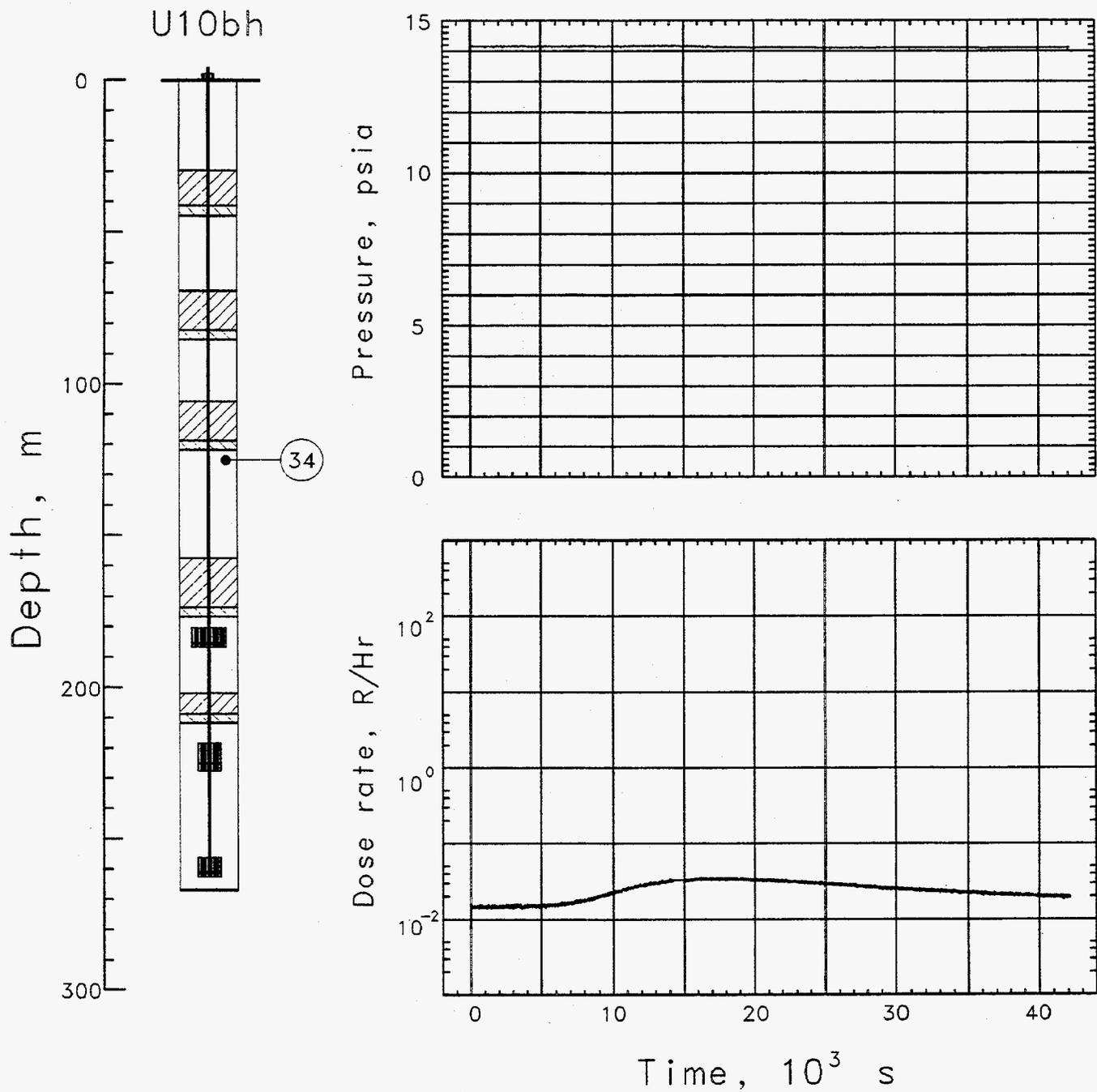
Figure 3.4 Pressure and radiation measured in the coarse stemming below SGC plug #3 (stations 34 at 122 m depth and 11 at 125 m depth). First arrival of radiation was at about 5000 s.
