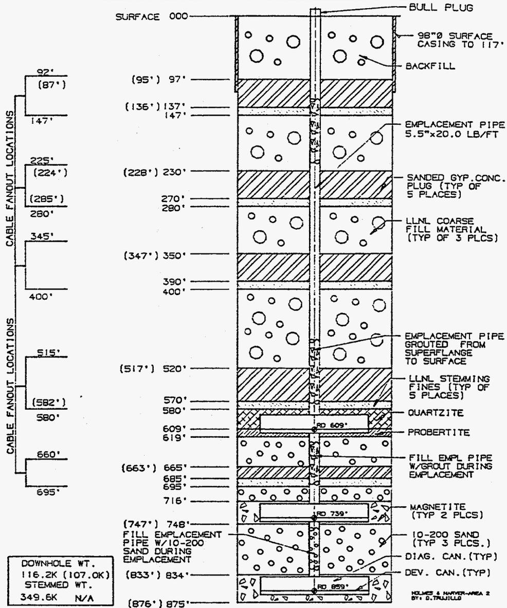
Figure 1.4 As-built stemming plan for hole U10bh.
