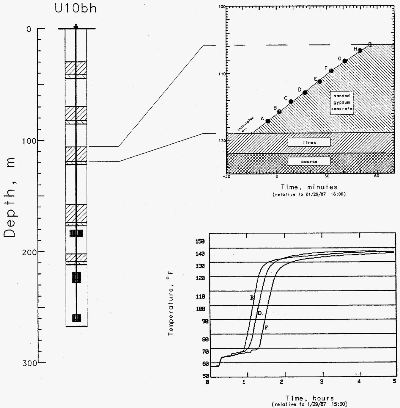
Figure 2.3 Sanded gypsum emplacement for plug #3. The upper and lower plug boundaries were calculated or determined with a tag line (open circle). Solid symbols indicate the probe elevations. Probes labeled B, D, and F included temperature sensors.
