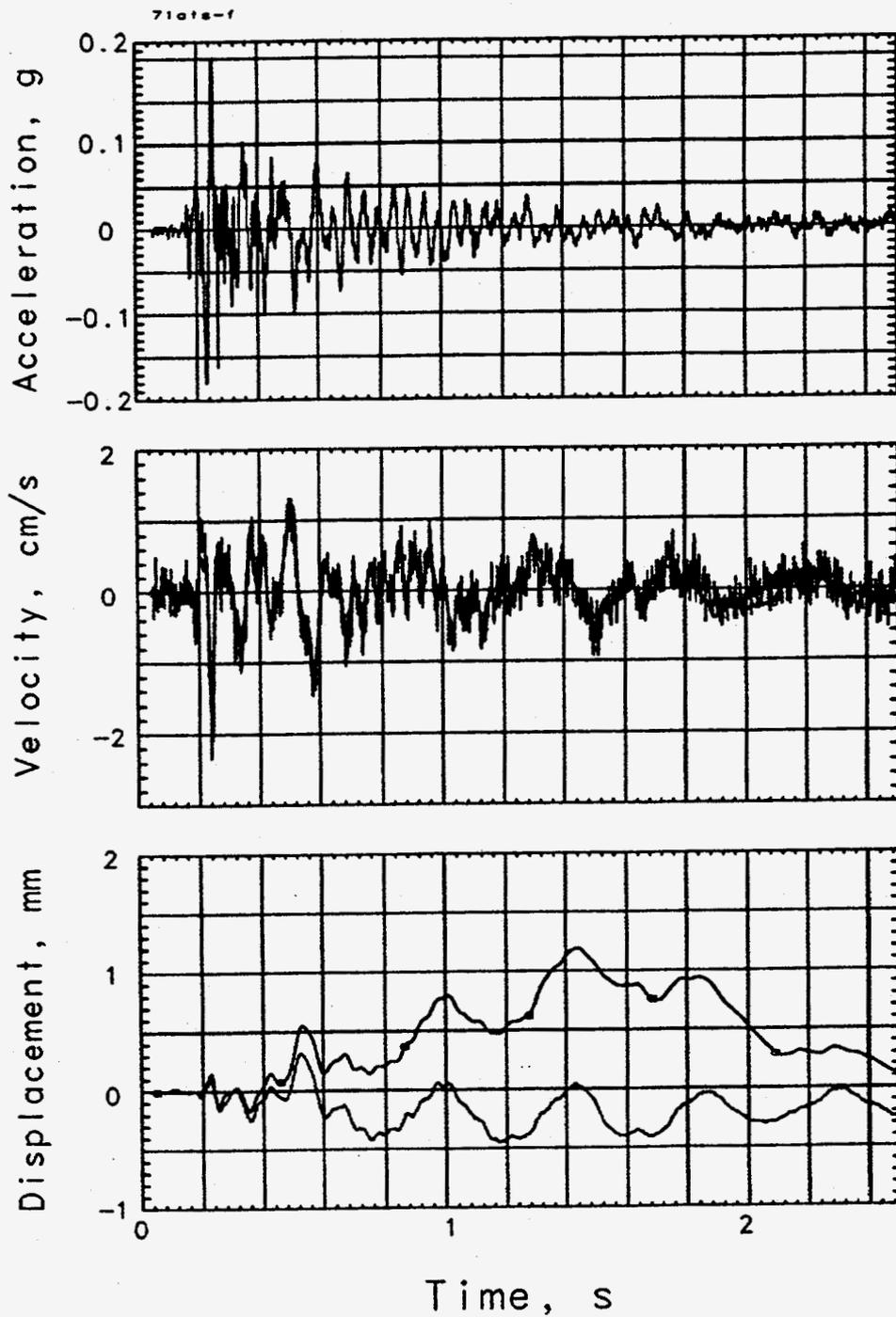
Figure 4.3 Explosion-induced horizontal-transverse motion of the recording trailer (station 71). Records annotated with an 'a' are derived from the accelerometer.
