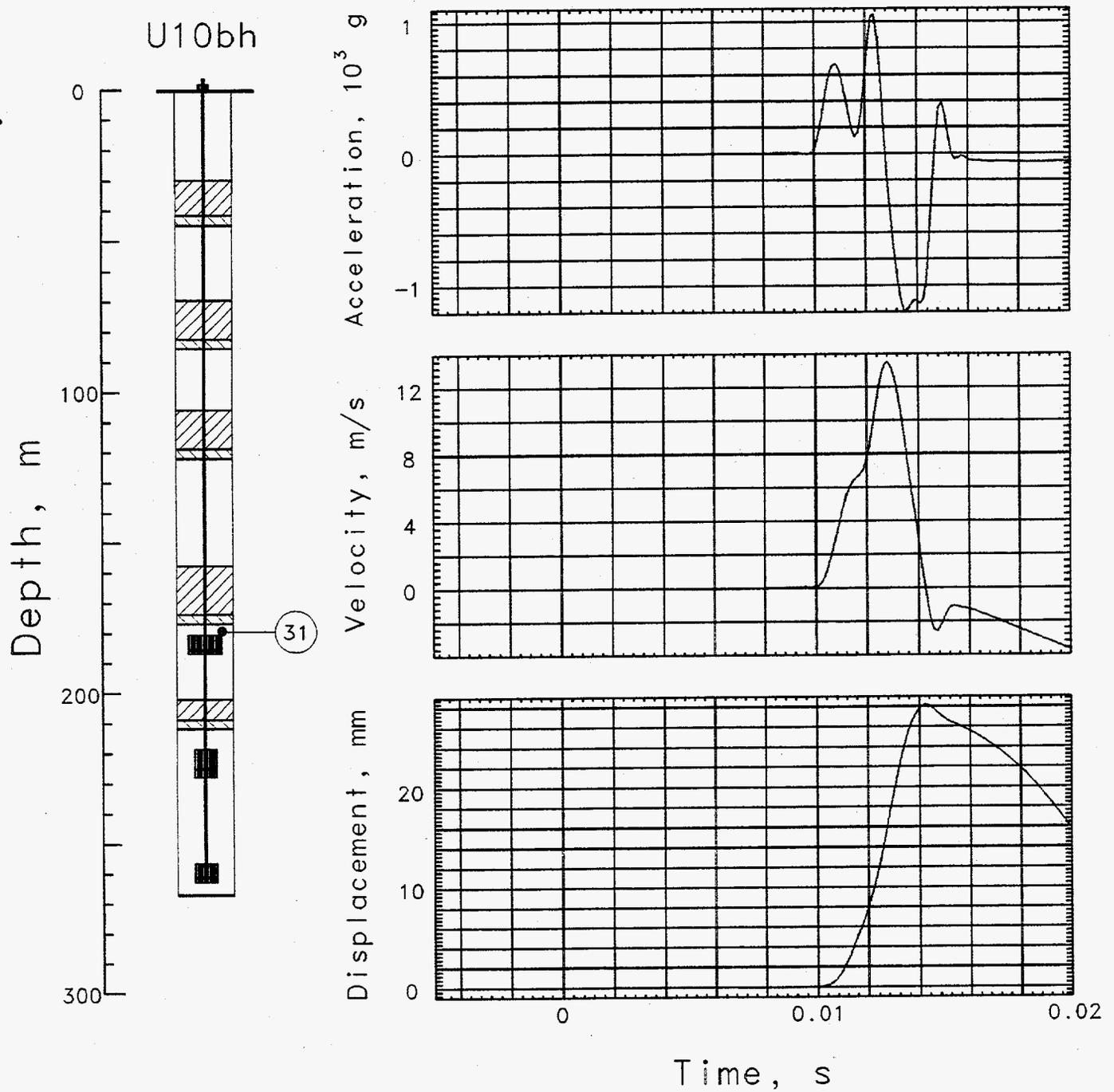
Figure 3.13 Explosion-induced vertical motion in the coarse stemming of the emplacement hole at a depth of 178 m (station 31, below plug #2). The transducer was apparently damaged at about 0.016 s.
