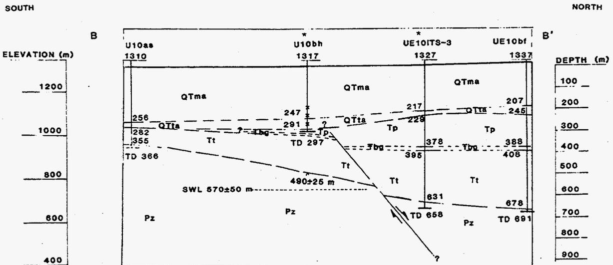
U10bh Geologic Cross Section B-B'
