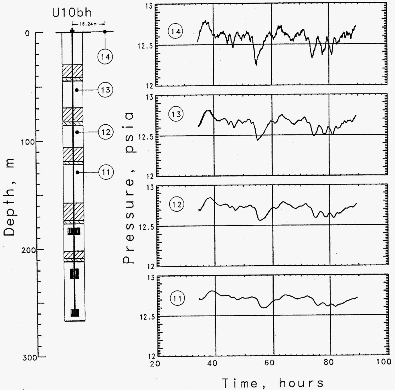
Figure 3.12 Pressures measured in the emplacement hole as a study of site permeability.
