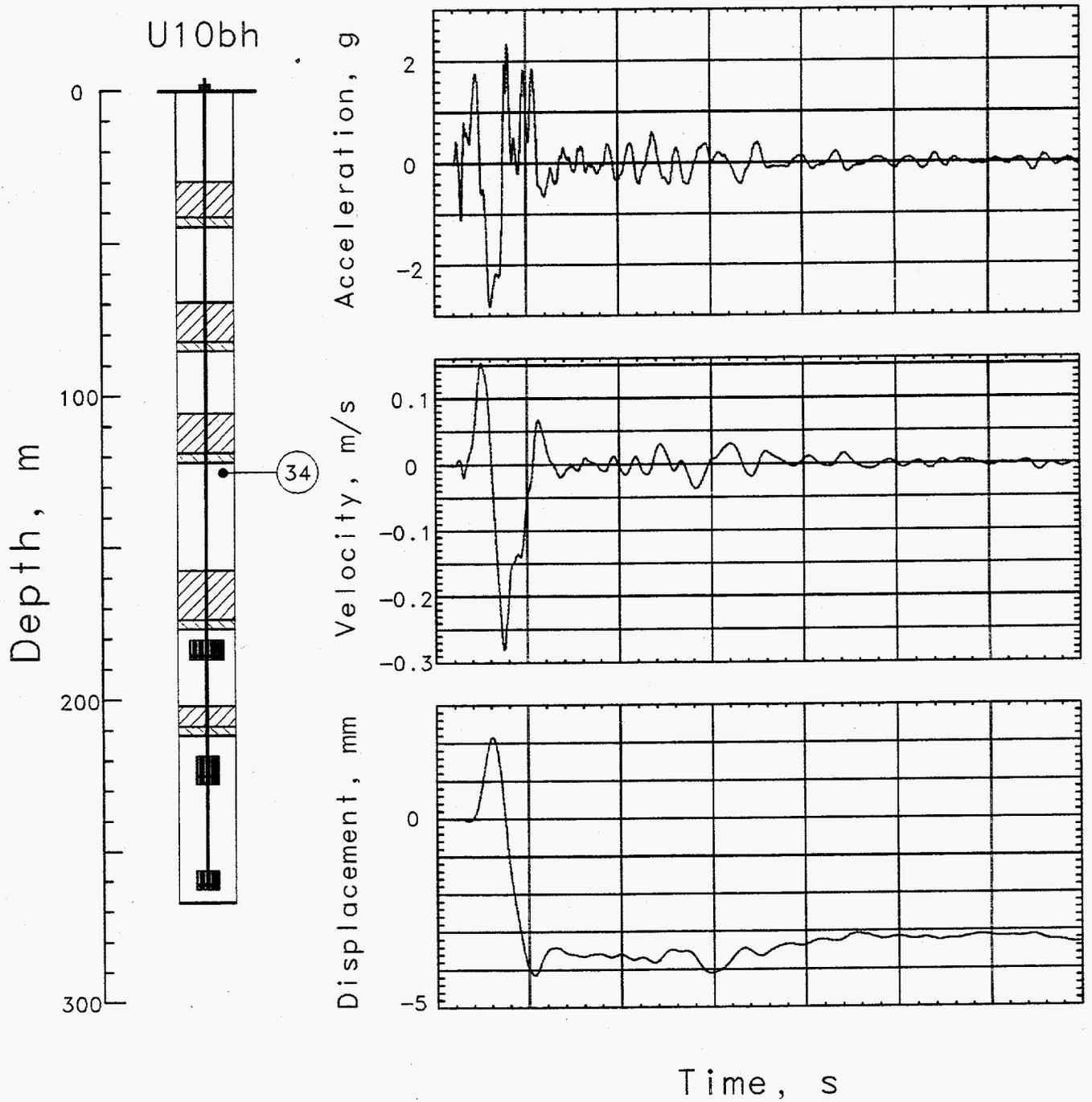
Figure 3.17 Explosion-induced vertical motion in the coarse stemming of the emplacement hole at a depth of 122 m (station 34, below plug #3).
