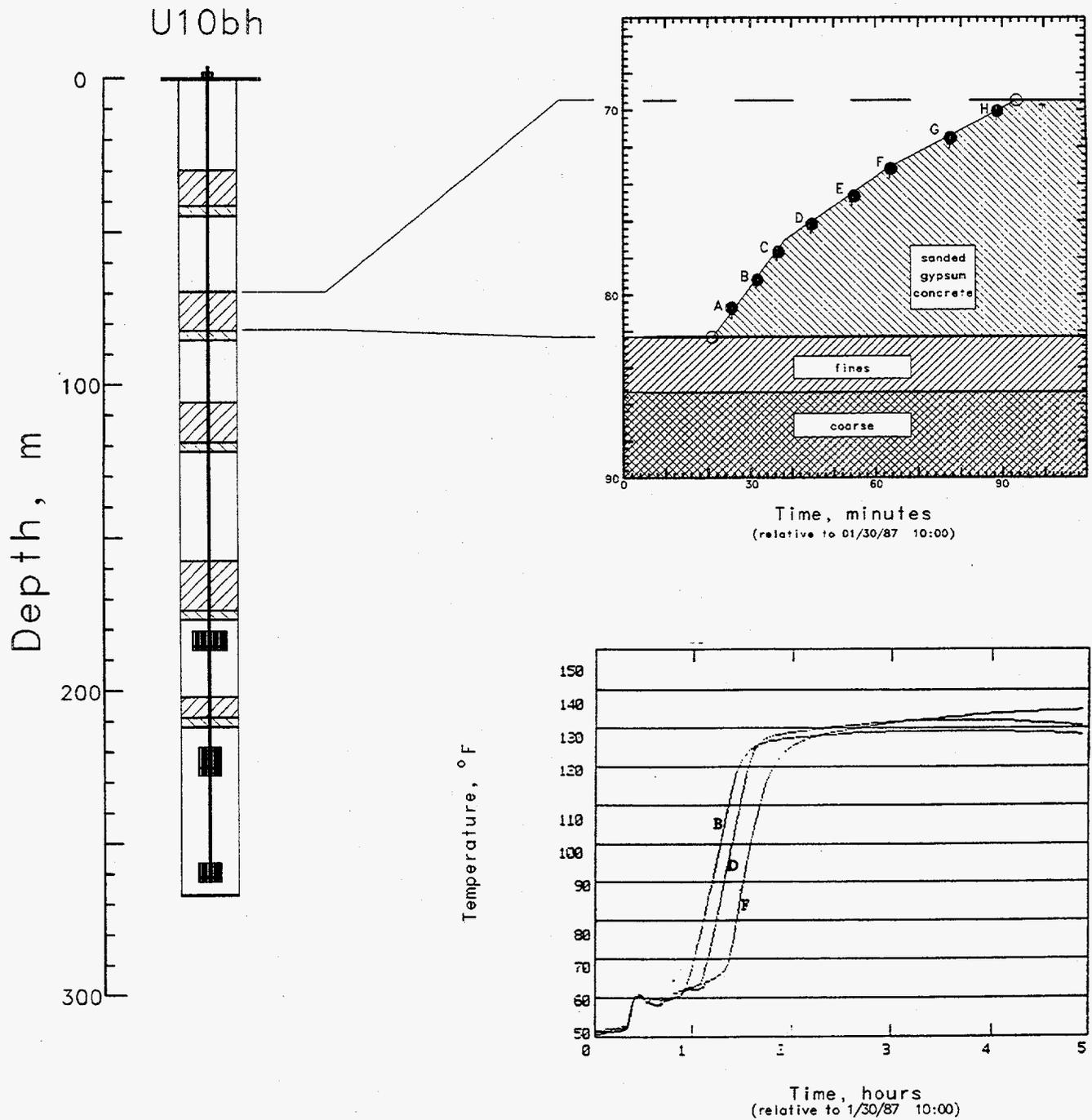
Figure 2.4 Sanded gypsum emplacement for plug #4. The upper and lower plug boundaries were determined with a tag line (open circles). Solid symbols indicate the probe elevations. Probes labeled B, D, and F included temperature sensors.
