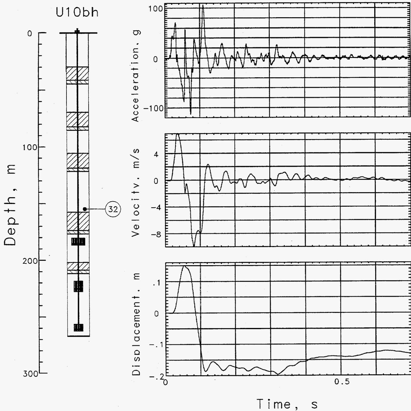
Figure 3.16 Explosion-induced vertical motion in the course of the emplacement hole at a depth of 152 m (station 32, above plug #2).
