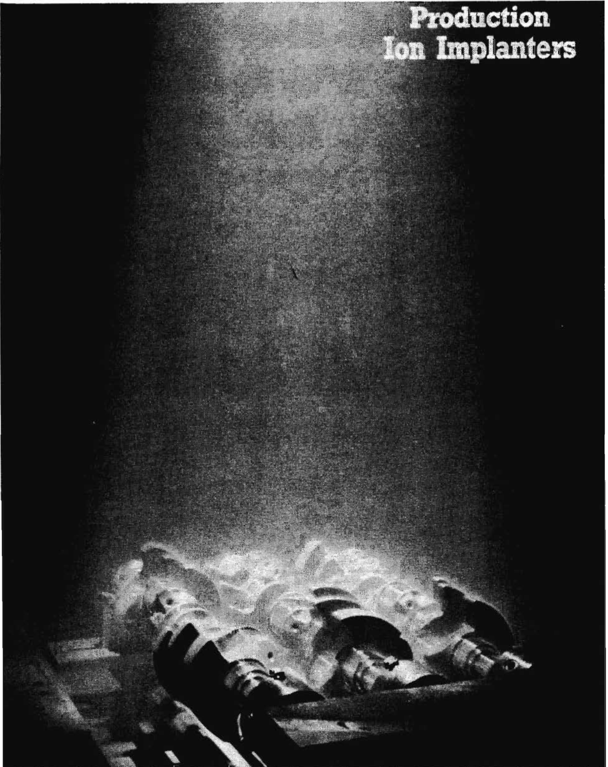
Figure 4. Automotive crankshafts undergoing N-ion implantation. The beam diverges as a cone from the source and is unanalyzed for mass, molecular, or charge content. This facility is at AEA Industrial Technology: Harwell Laboratory, United Kingdom. (Photograph courtesy of G. Dearnaley.)
