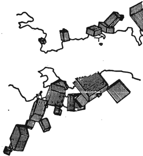
Figure 7. Buildup of localized chains in preference to homogenous distribution of sodium chloride aerosol (Watson, as cited in Reference 16)
