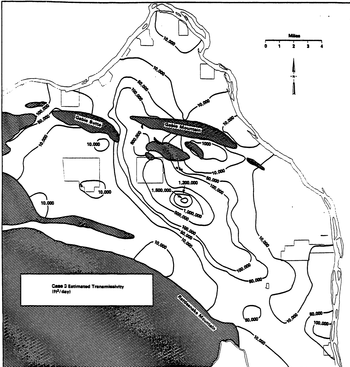
FIGURE A.29. Distribution of Transmissivities from Case 3 of the Inverse Application (from Jacobson and Freshley 1990)
