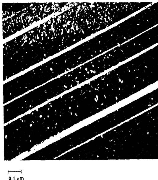
Figure 7(b). Deformation twins in ion-irradiated 304L SS, deformed 10% at room temperature.
