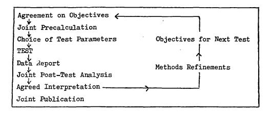
The design stage of experiments within this sequence needs careful consideration because there are limitations on the match that can be achieved between a test rig and the conditions within a real fast reactor.
