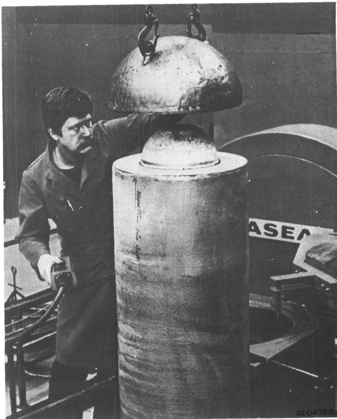
Figure 4. Encapsulating Simulated Spent Fuel in Ceramic (ASEA)
