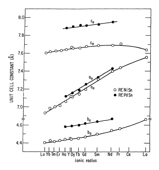
Fig. 1. Unit cell constants vs ionic radii for R.E. Ni(Pd)Sn compounds.
