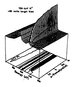
Figure 1: A joint distribution of 0° electrons showing energy spectra for various levels of microwave power (watts). The lower-energy peak, unaffected by microwave power, is caused by convoy electrons. The higher-energy peak, which grows with power, is produced by field-ionization of Rydberg atoms in the microwave cavity. At low power, there is an additional contribution from atoms ionizing in the spectrometer field (170 v/cm).
