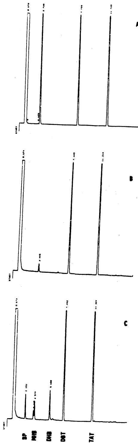
Figure 1. Gas Chromatography Analysis. Panel A: Uninoculated Control; Panel B: Strain DK6' incubated with DBT in M9 Glycerol medium; Panel C: Same as Panel B except spiked with three biphenyl standards. BP-Biphenyl, MHB--2-hydroxybiphenyl, DHB--2,2'-dihydroxybiphenyl, TAT--thianthrene.
