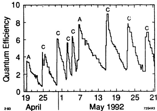
Figure 4. Quantum efficiency (750 nm and 120 kV) for first two activation cycles at the SLC injector. "A" indicates activation (heat cleaning/cesiation/fluoride), "C" indicates cesiation only. The initial QE had dropped to ~3.5% by the time the plot began.
