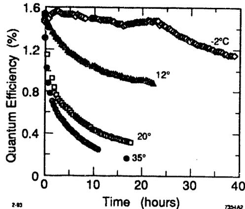
Figure 2. Temperature dependence of photocathode quantum efficiency lifetime.
