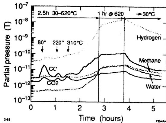
Figure 3. Partial pressures in the gun during cathode heat cleaning as measured with a VG Sensorlab RGA system.
