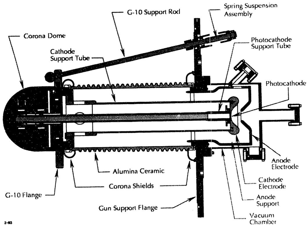
Figure 1. SLC photocathode diode gun. (See Ref. 3.)
