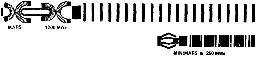
Fig. 9. Minimum adiabatic length plugs ( \cong 8 m) allows smaller reactors (Minimars) compared to MARS.
