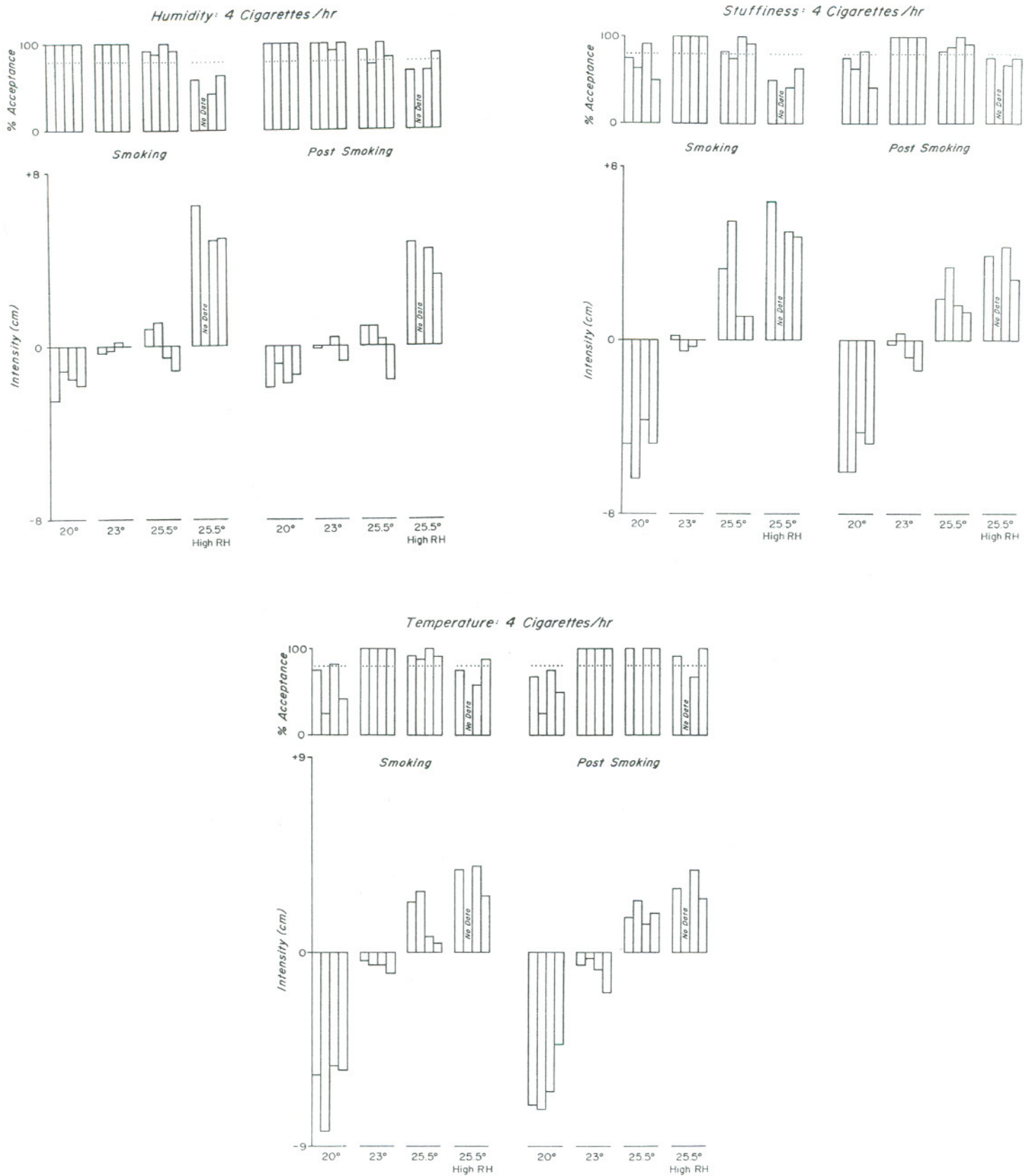
Fig. 26. Showing how occupants (smokers) rated the magnitude and acceptability of humidity, stuffiness, and temperature during smoking of 4 cigarettes per hour and during post-smoking segments. In each group of 4 bars, ventilation rate varies from left to right as follows: 11 cfm ( 5.5 \text{ L}\cdot\text{s}^{-1} ) per occupant, 25 cfm ( 12.5 \text{ L}\cdot\text{s}^{-1} ), 35 cfm ( 17.5 \text{ L}\cdot\text{s}^{-1} ) and 68 cfm ( 34 \text{ L}\cdot\text{s}^{-1} ) per occupant.
