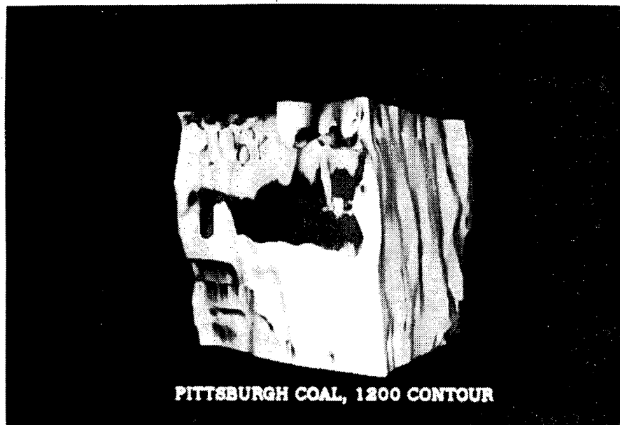
Figure 11-1. Three-dimensional image of isodensity contours on Pittsburgh #8 coal. Density set at 1200 CT numbers.
