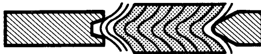
SPIRAL WOUND GASKET WITH INNER AND OUTER RINGS FOR CENTERING AND COMPRESSION LIMITING.
