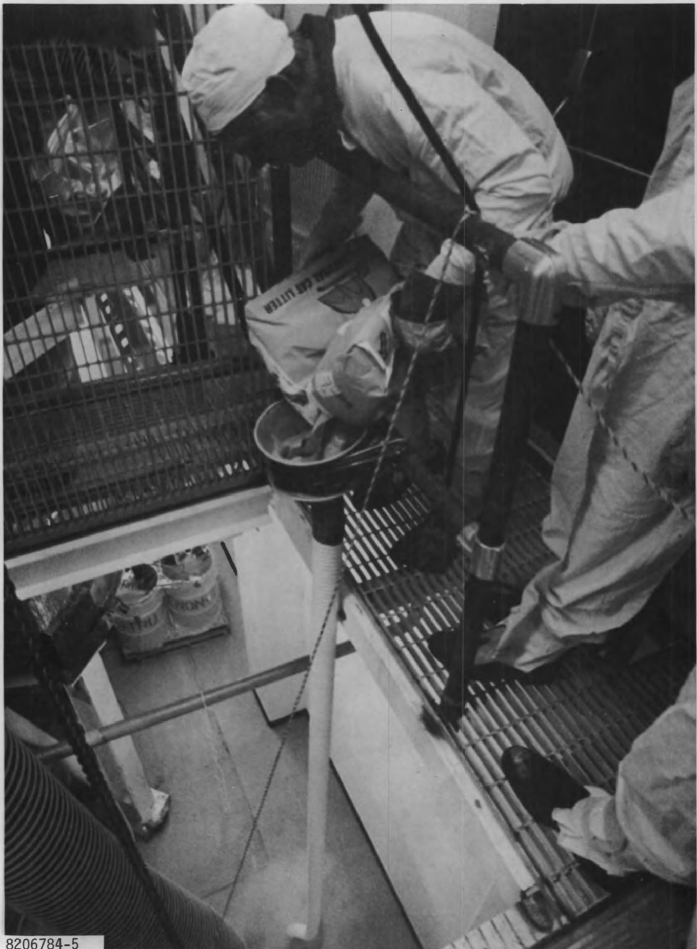
FIGURE 3-22. Remote Addition of Adsorbant Material
