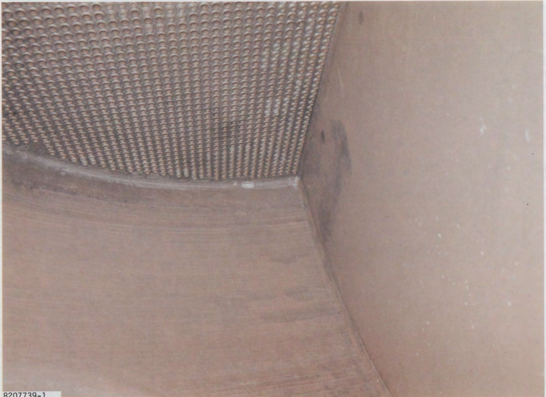
FIGURE 4-11. Hot Leg Surfaces After the NP/LOMI Process
