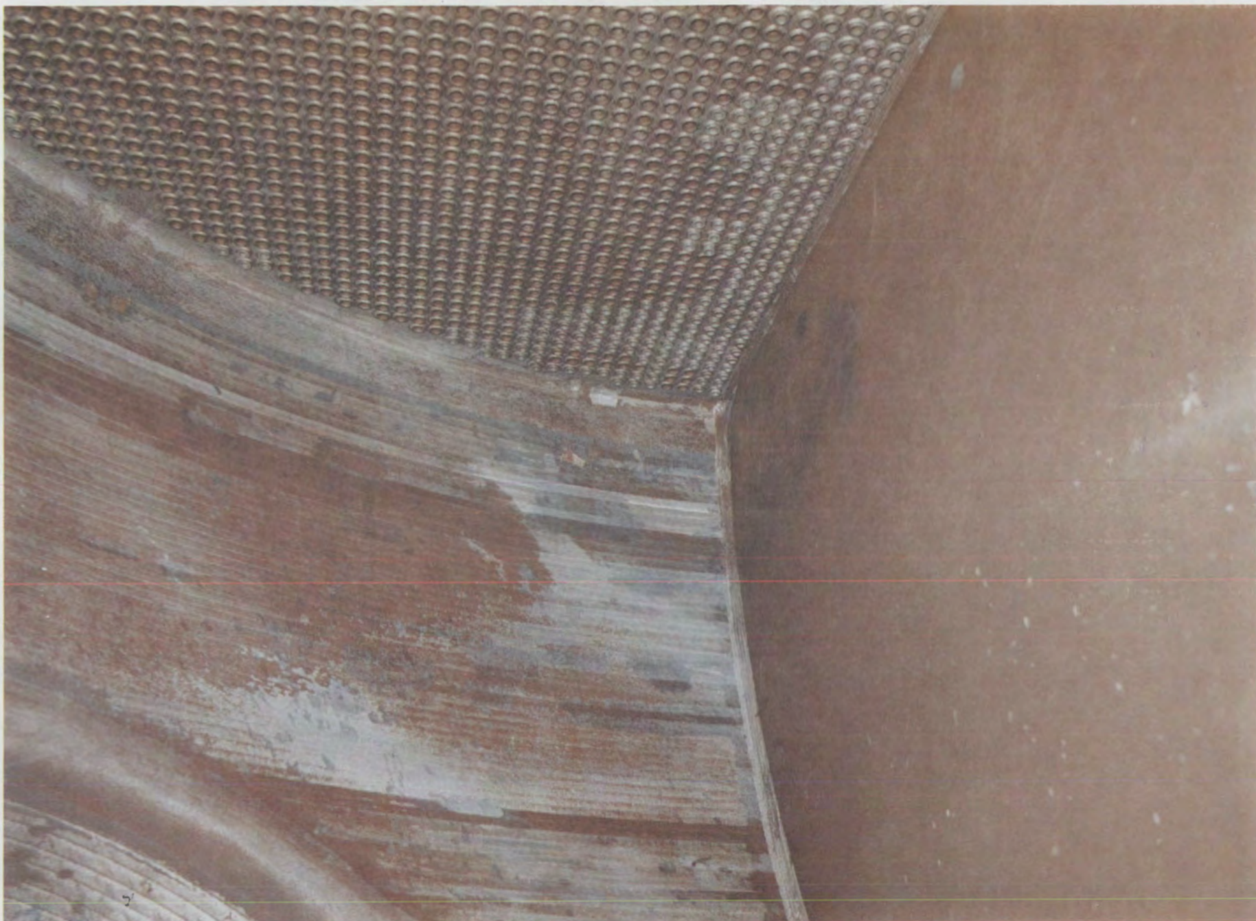
FIGURE 4-12. Hot Leg Surfaces After the AP/POD Process
