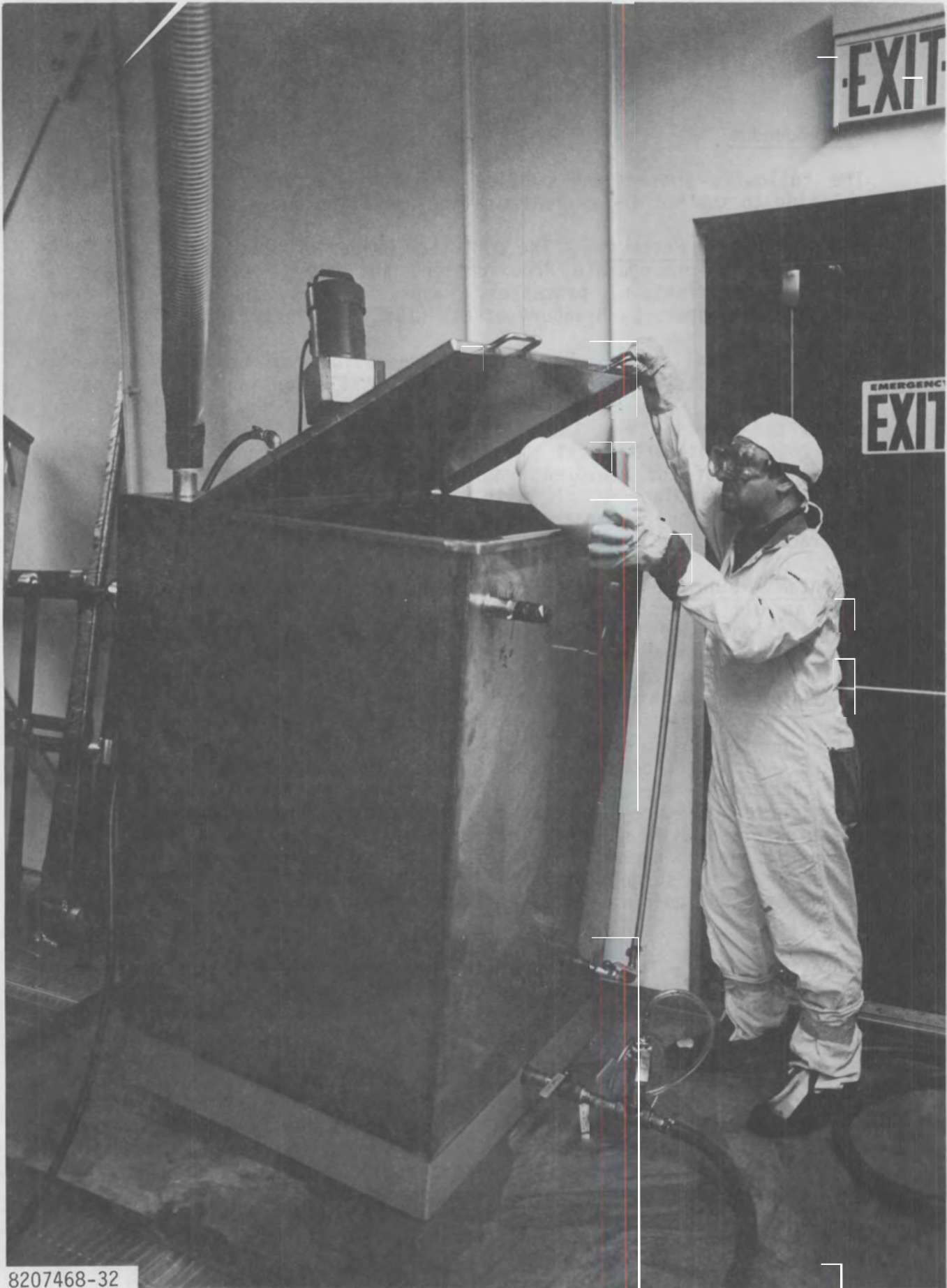
FIGURE 4-1. Chemical Addition/Mixing Tank for Hot Leg Decontamination
