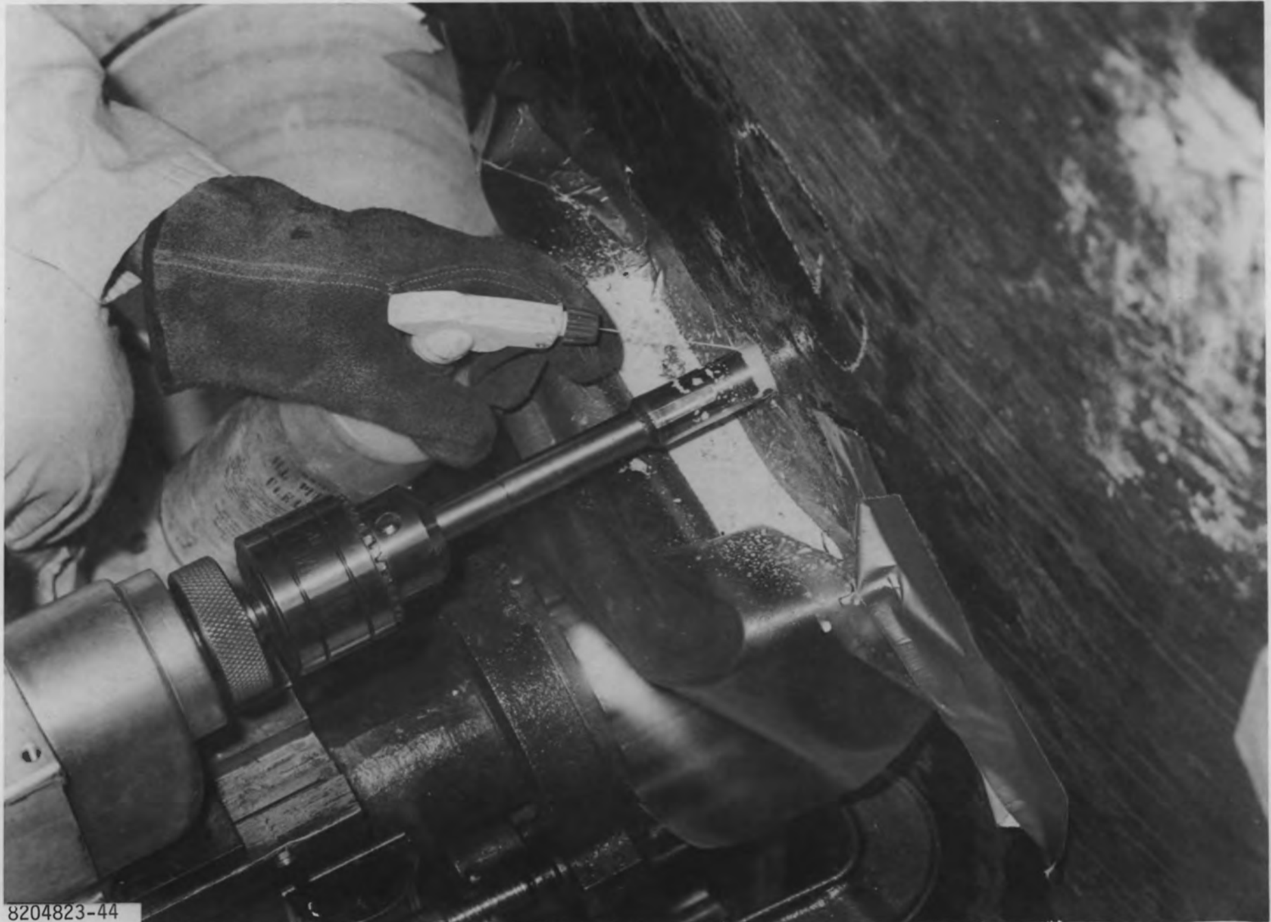
FIGURE 2-1. Core Drilling to Obtain Samples of the Interior Channel Head Surfaces
