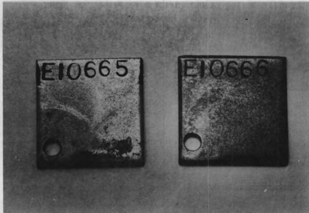
FIGURE 6-13. Prefilmed Corrosion Coupons After the Hot Leg Decontamination
