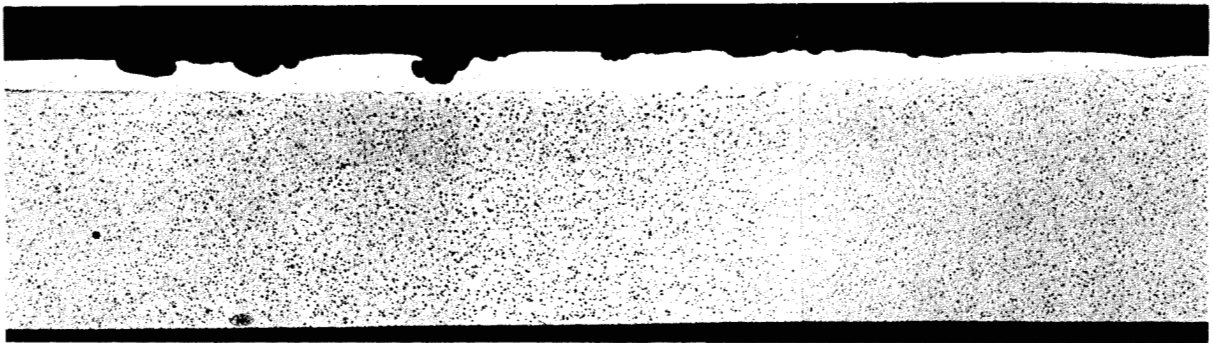
b) 80% W Sintered 1 h at 1470°C 98.1% of 15.43 g/cm 3 (8X)
