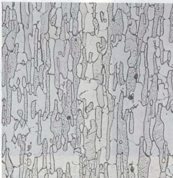
As-Sintered at 1435°C for 20 h--22-aA 14.0 g/cm 3 . Hardness HRC 22
