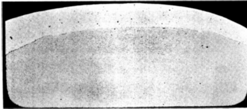
a) 70% W Sintered 1 h at 1475°C 101.0% of 14.03 g/cm 3 (6.65X)
