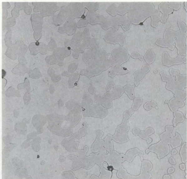
As-Sintered at 1435°C for 20 h--22-aA 14.0 g/cm 3 . Hardness HRC 22
