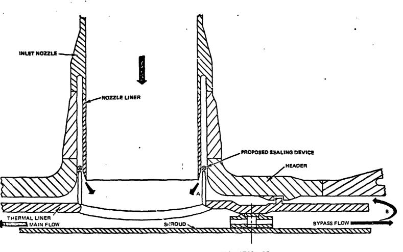
FIGURE 10. REVISED CONFIGURATION OF INLET NOZZLE REGION
