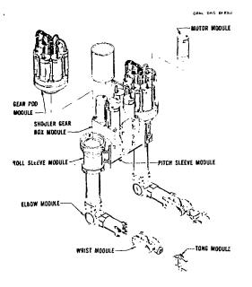
Fig. 5. Advanced servomanipulator modularization
