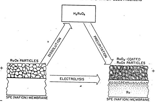
MECHANISM OF PERFORMANCE DEGRADATION WITH TIME FOR OXYGEN EVOLUTION ON RUOX ELECTRODES IN SPE WATER ELECTROLYZERS
