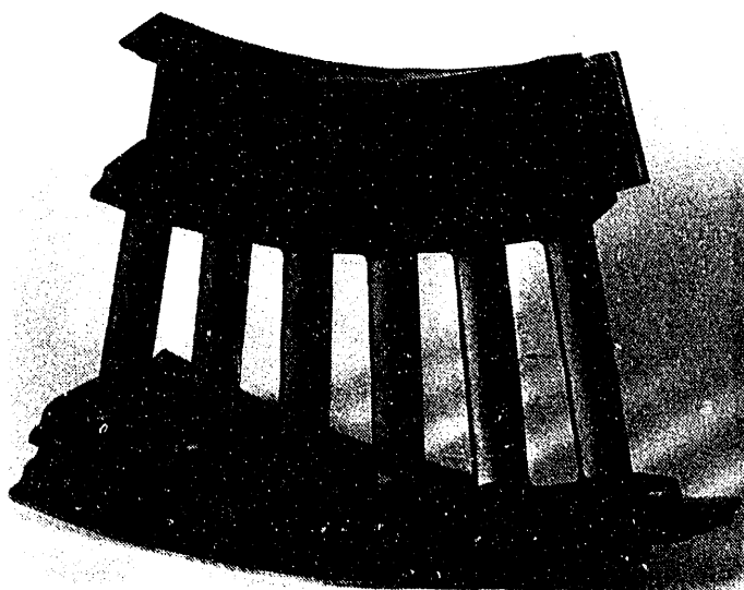
Figure 5. Second Stage Vane Segment After Water Washing
