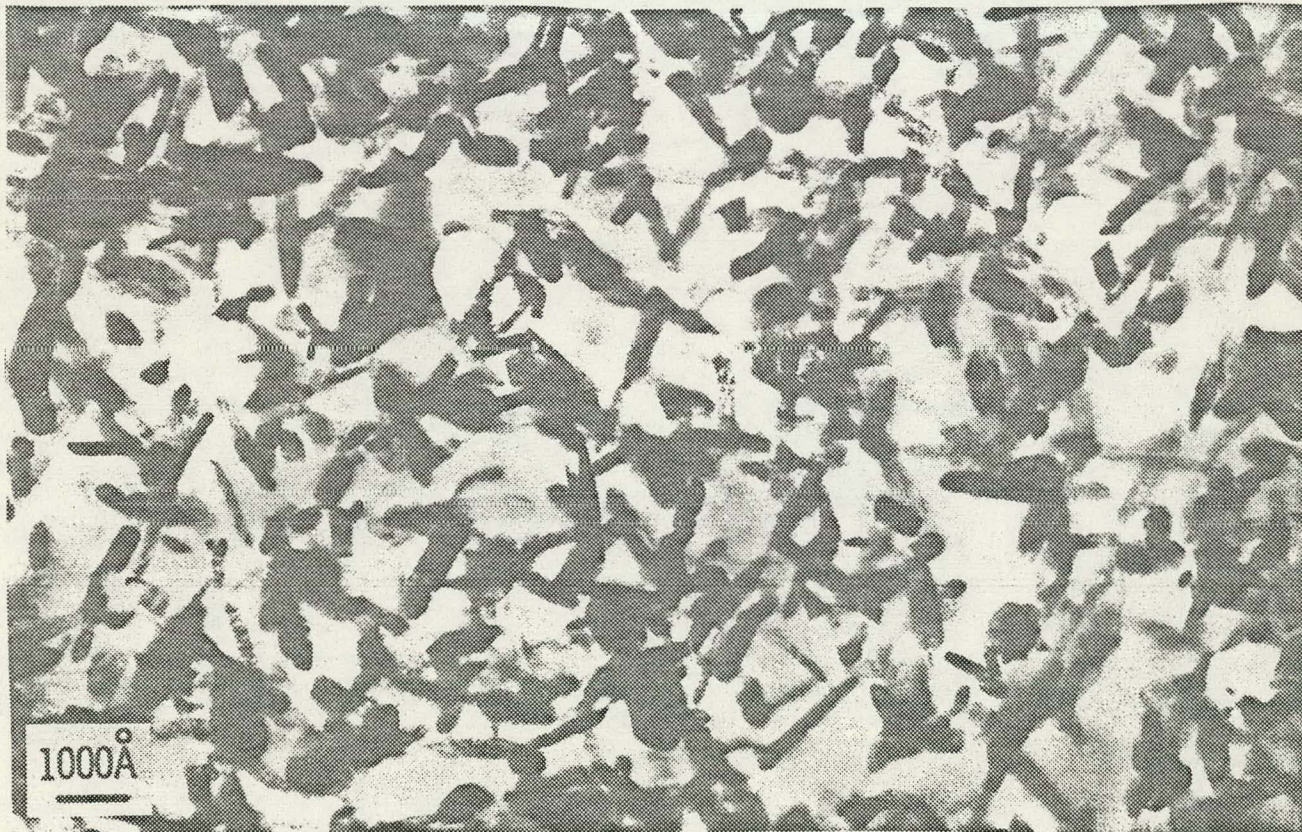
Fig. 6 - Precipitate microstructure in the 2% silicon alloy after irradiation at 610°C to a fluence of 3.5 \times 10^{22} n/cm 2 (imaged with 1.0 MeV electrons).
